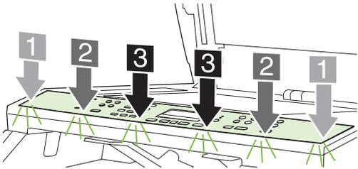
**Figure 5-19** Replace the control-panel bezel (3 of 3)
