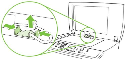
**Figure 5-3** Replace the ADF (2 of 6 )
