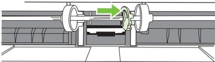
Moving the roller cam will reveal a pin in the roller shaft. Do not remove the pin.
