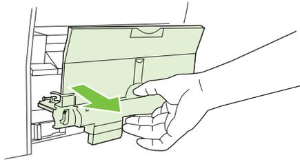
**CAUTION** The parts on the internal surface of the fuser assembly are very hot. To avoid burning yourself, do not touch those parts.
