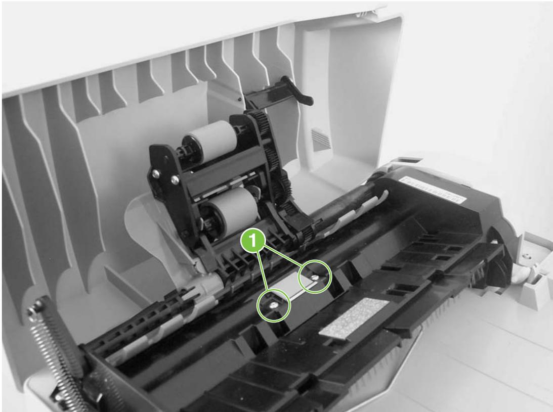
**Figure 5-14** Remove the ADF separation pad (2 of 2)
