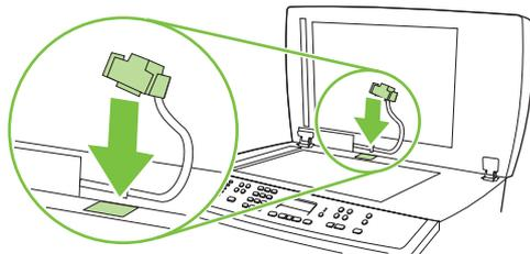
**Figure 5-7** Replace the ADF (6 of 6 )
