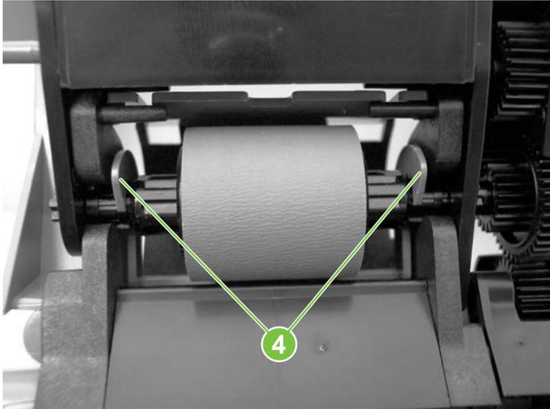
**Figure 5-12** Remove the ADF pickup-roller assembly (5 of 5)
