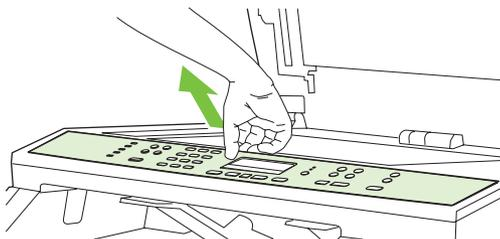
**Figure 5-17** Replace the control-panel bezel (1 of 3)
