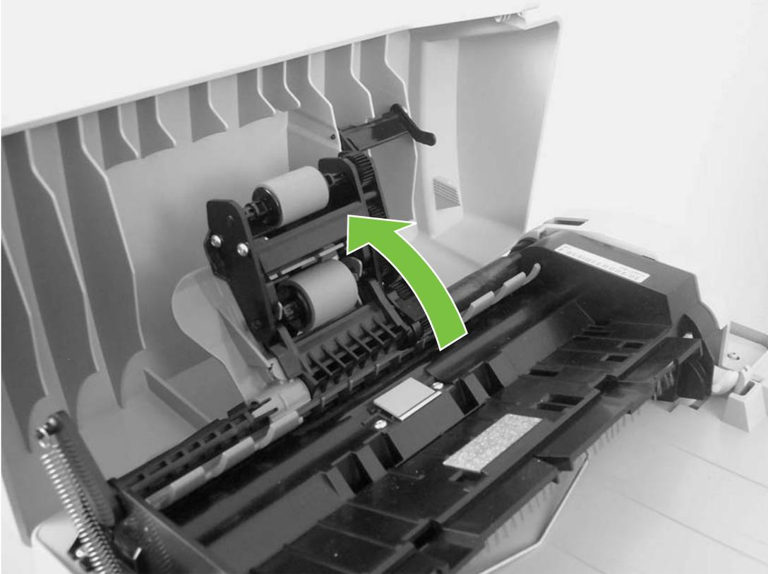
**Figure 5-13** Remove the ADF separation pad (1 of 2)
