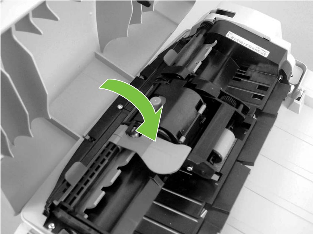
**Figure 5-11** Remove the ADF pickup-roller assembly (4 of 5)
