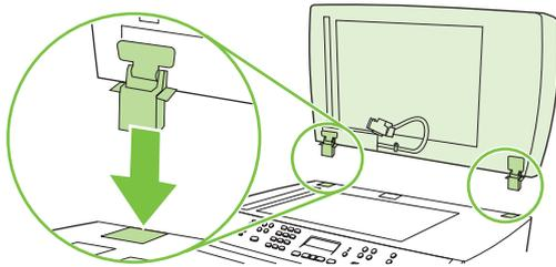
**Figure 5-6** Replace the ADF (5 of 6 )
