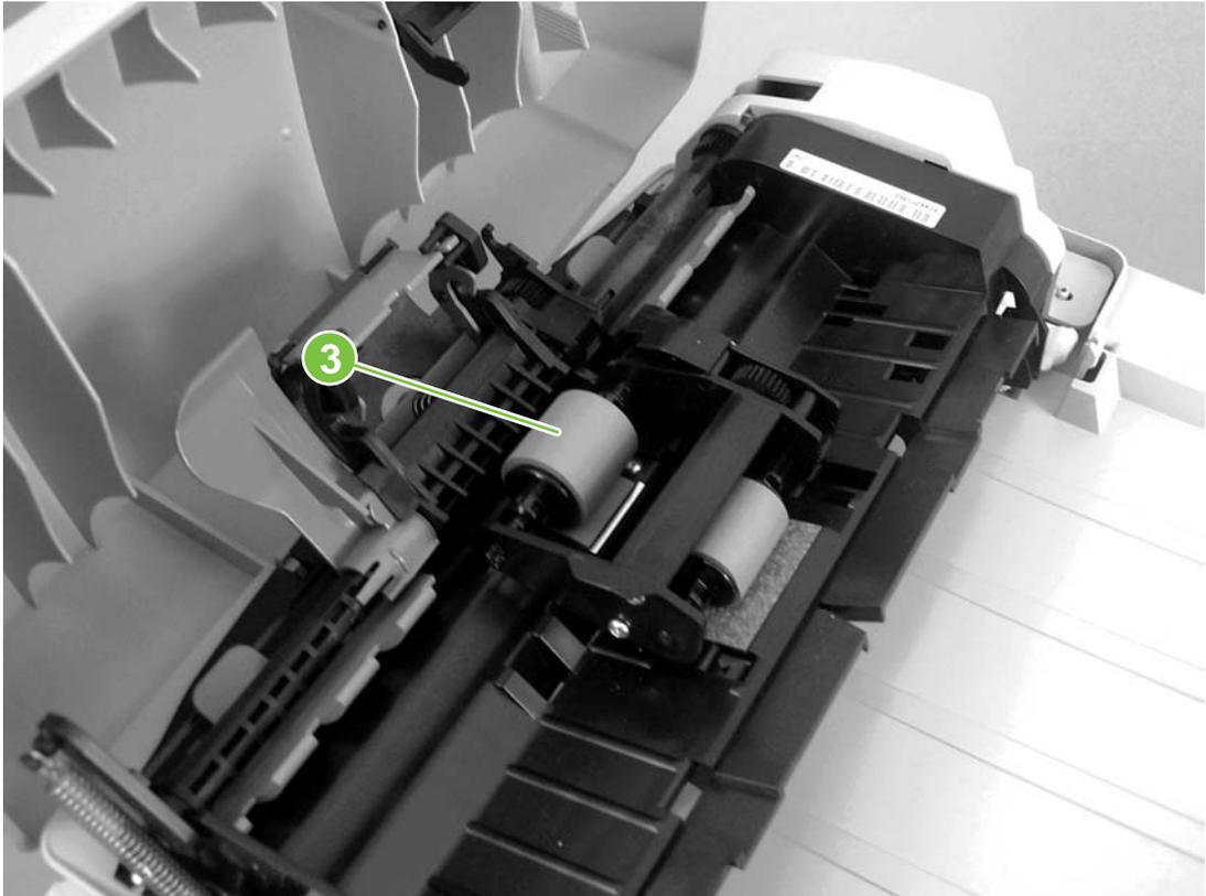
**Figure 5-10** Remove the ADF pickup-roller assembly (3 of 5)
