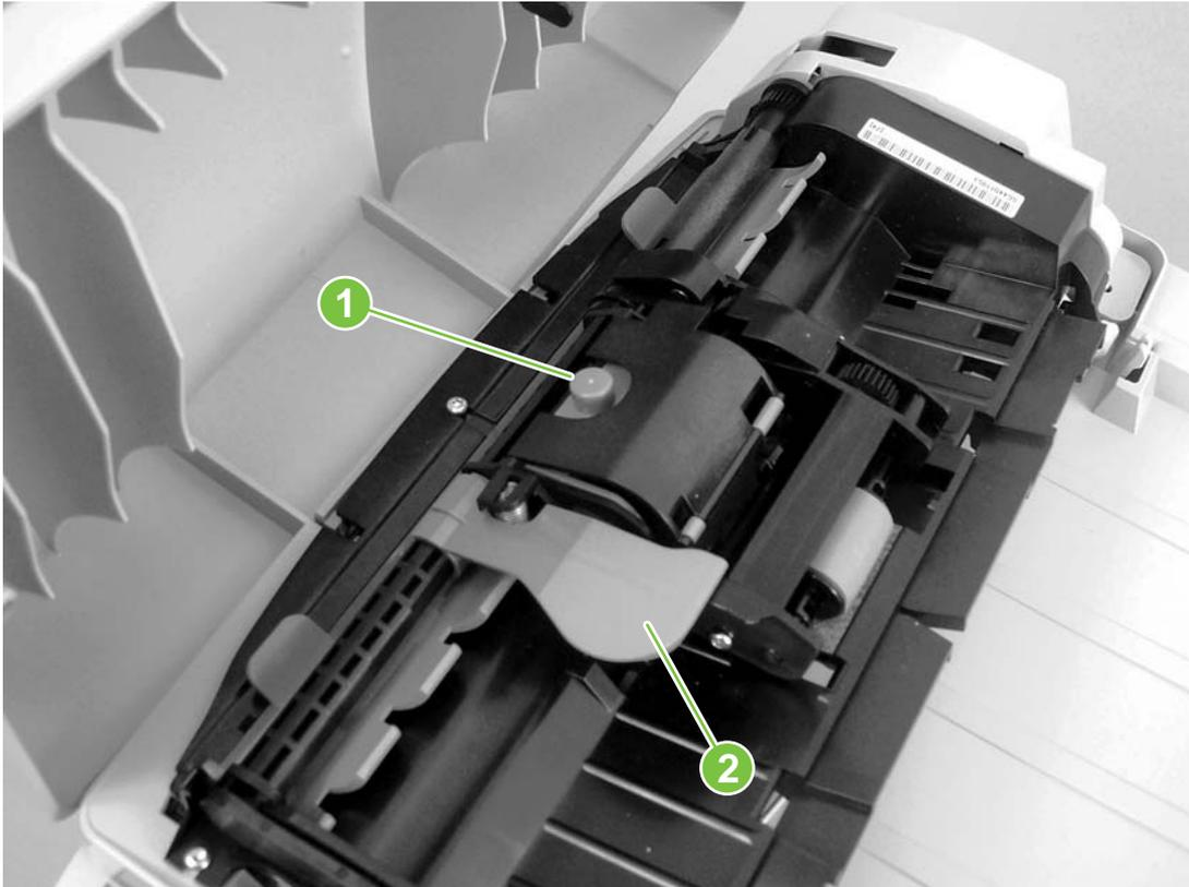
**Figure 5-9** Remove the ADF pickup-roller assembly (2 of 5)
