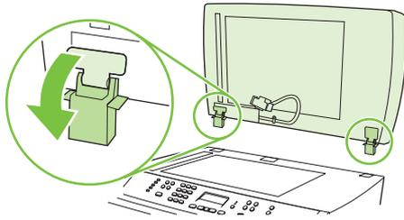
**Figure 5-5** Replace the ADF (4 of 6 )
