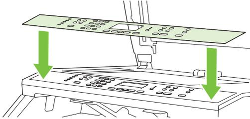
**Figure 5-18** Replace the control-panel bezel (2 of 3)
