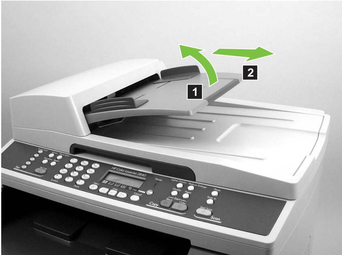
**Figure 5-8** Remove the ADF pickup-roller assembly (1 of 5)
