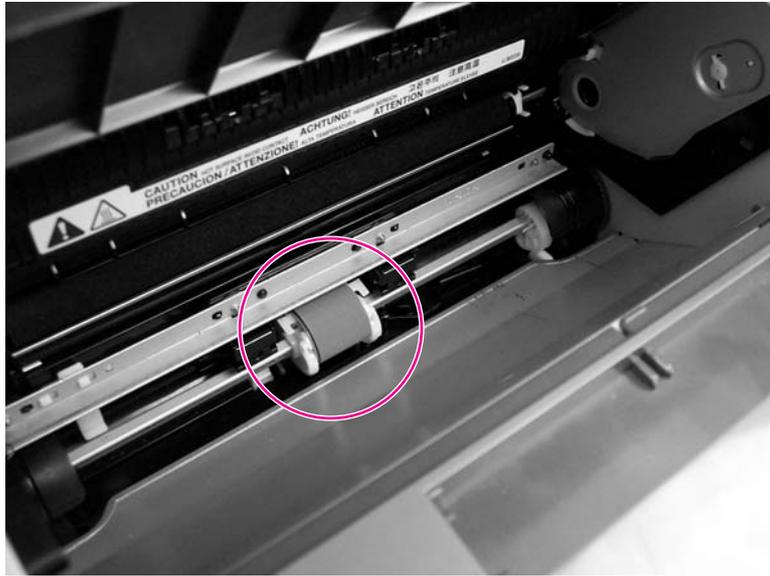
**Figure 5-93.** Remove the printer pickup roller (1 of 5)
