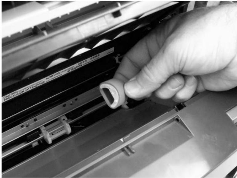
**Figure 5-95.** Remove the printer pickup roller (3 of 5)
