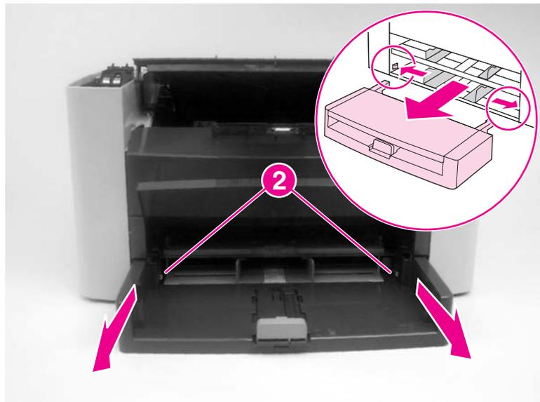
**Figure 5-100.** Remove the media input tray (3 of 3)
