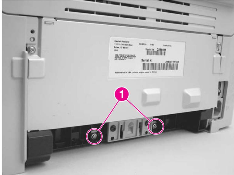
**Figure 5-89.** Remove the printer separation pad (1 of 2)
