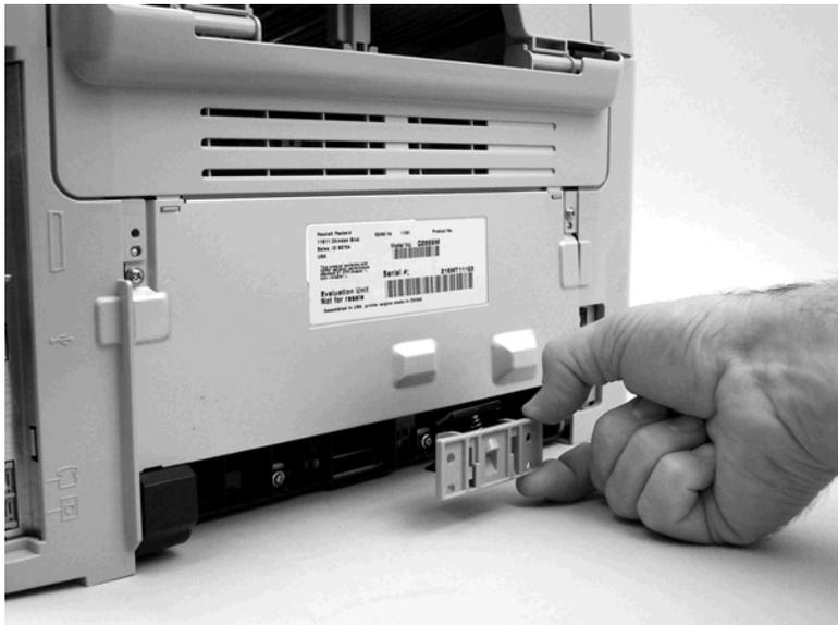
**Figure 5-90.** Remove the printer separation pad (2 of 2)
