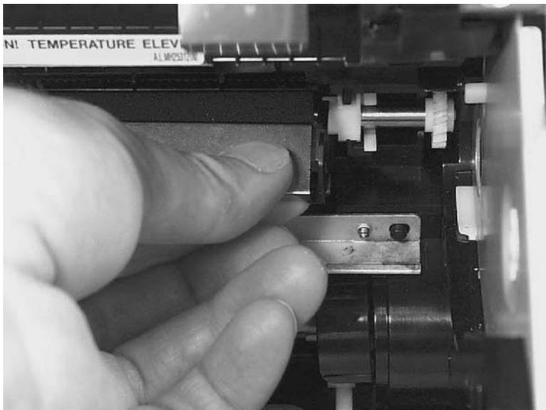
**Figure 5-102.** Remove the transfer roller (2 of 3)
