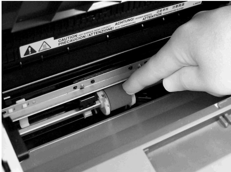
**Figure 5-97.** Remove the printer pickup roller (5 of 5)
