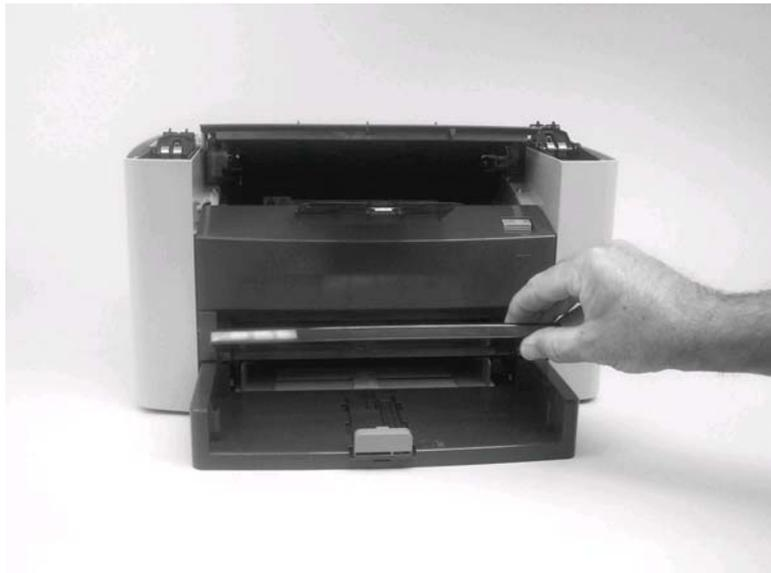
**Figure 5-98.** Remove the media input tray (1 of 3)
