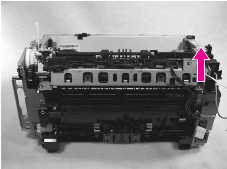
**Figure 5-144.** Remove the fuser assembly (2 of 2)
