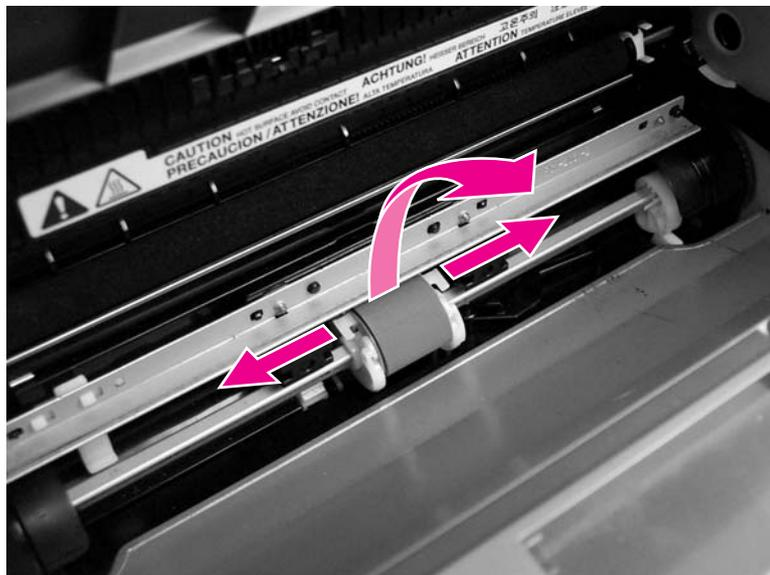
**Figure 5-94.** Remove the printer pickup roller (2 of 5)
