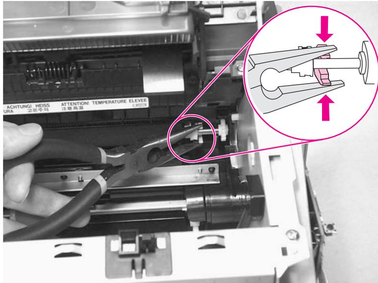
**Figure 5-103.** Remove the transfer roller (3 of 3)
