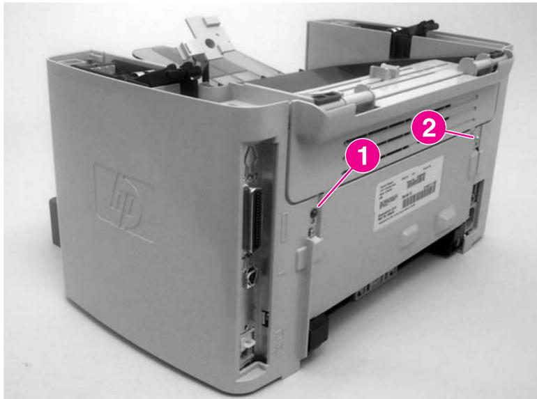
**Figure 5-104.** Remove the printer side covers (1 of 3)
