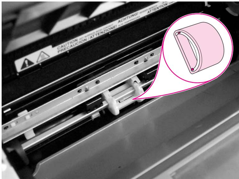
**Figure 5-96.** Remove the printer pickup roller (4 of 5)
