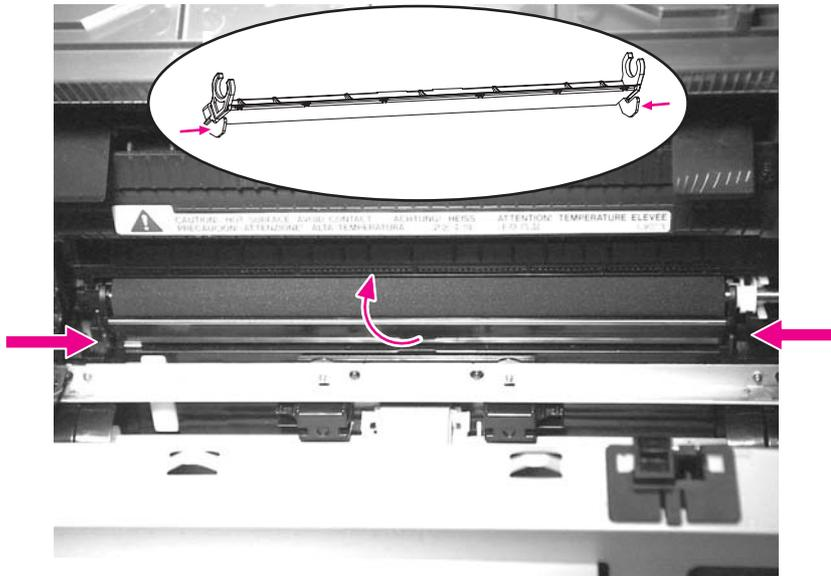
**Figure 5-101.** Remove the transfer roller (1 of 3)
