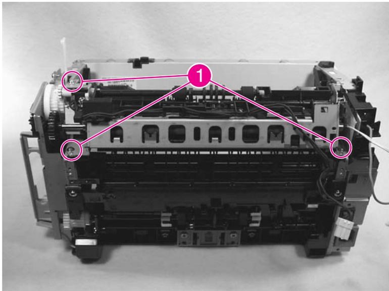
**Figure 5-143.** Remove the fuser assembly (1 of 2)
