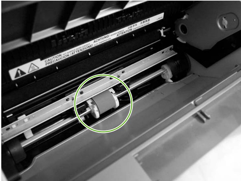
Figure 5-90 Removing the printer pickup roller (1 of 5)
