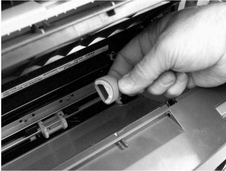
Figure 5-92 Removing the printer pickup roller (3 of 5)
