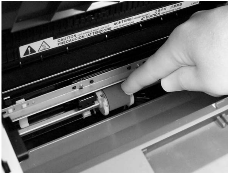
Figure 5-94 Removing the printer pickup roller (5 of 5)
