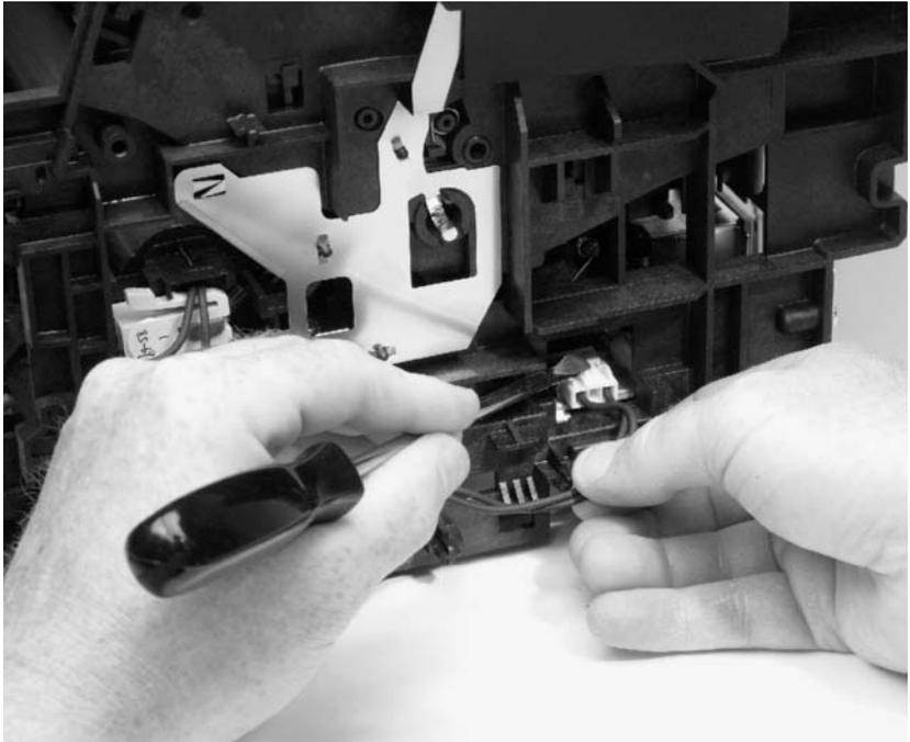
**Figure 50.** Fusing element removal (3 of 4)
