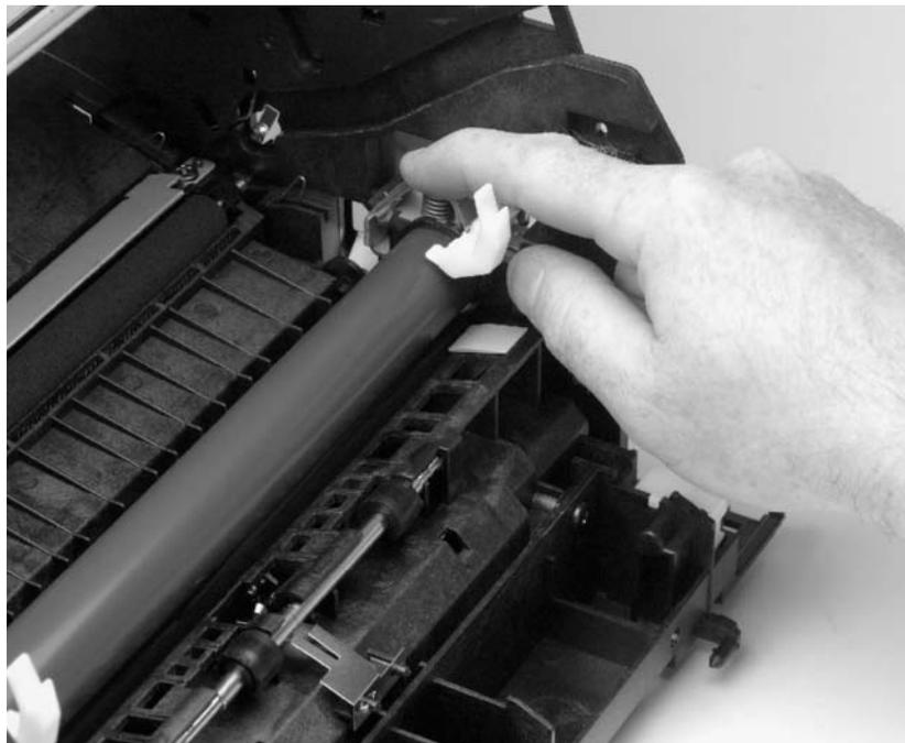
**Figure 48.** Fusing element metal clips reinstallation
