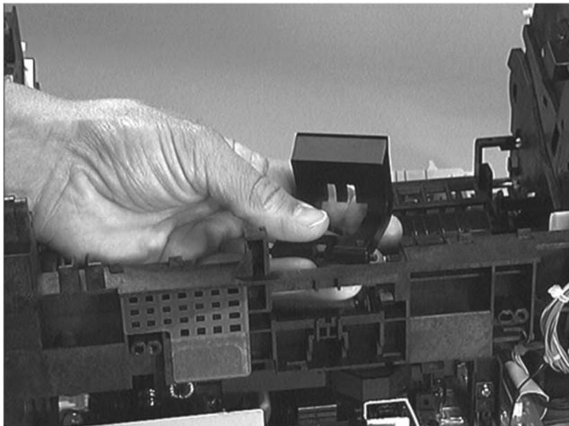
**Figure 63.** Separation pad removal (2 of 2)
