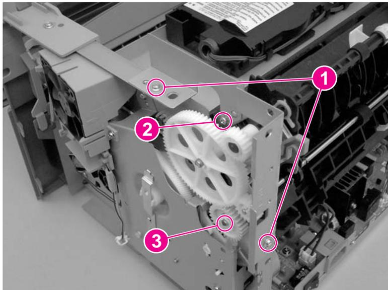
**Figure 5-64.** Remove the fuser assembly (1 of 4)
