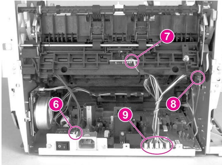
**Figure 5-67.** Remove the fuser assembly (4 of 4)
