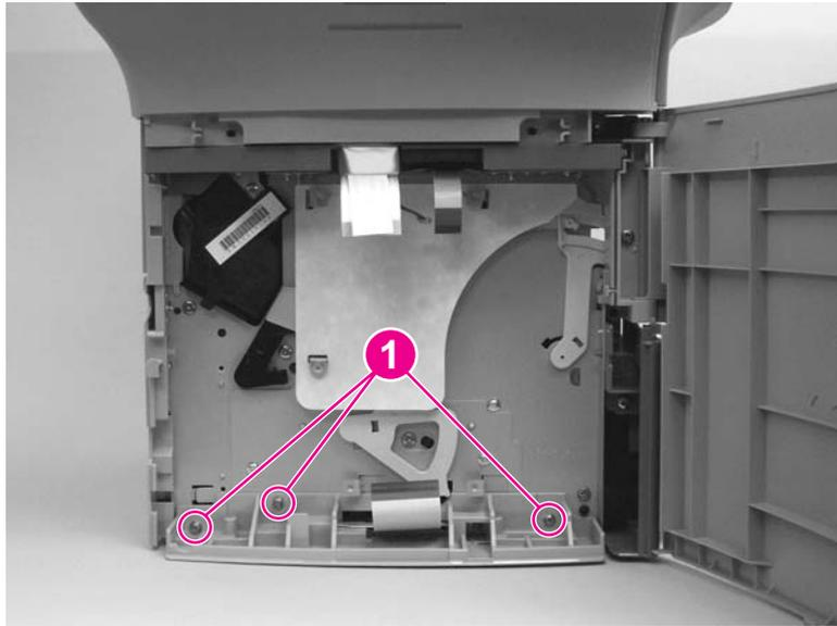
**Figure 5-63.** Remove the left bottom frame support
