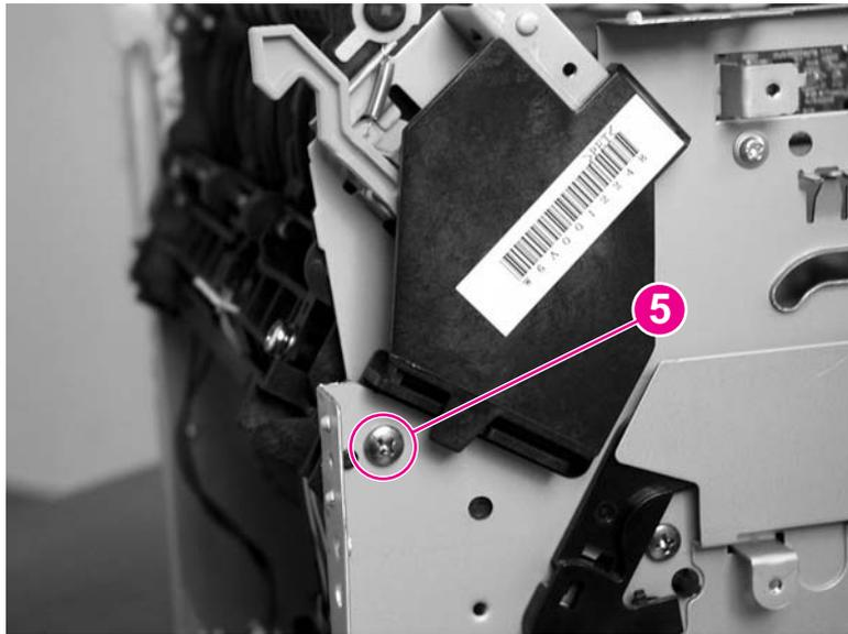
**Figure 5-66.** Remove the fuser assembly (3 of 4)
