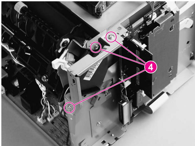
**Figure 5-65.** Remove the fuser assembly (2 of 4)
