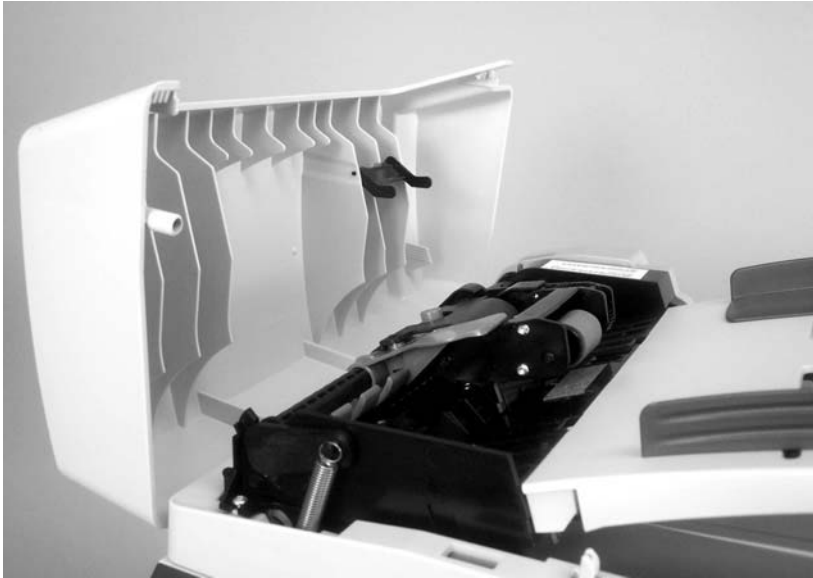
Figure 5-19 Replacing the ADF pickup-roller assembly (1 of 6)
