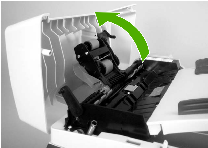
Figure 5-21 Replacing the ADF pickup-roller assembly (3 of 6)
