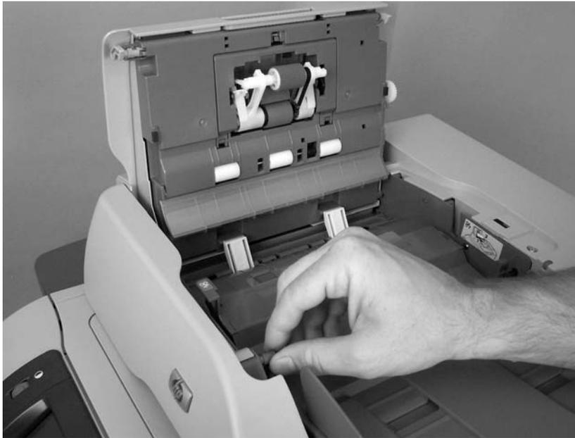
**Figure 5-6** Remove the ADF input tray (2 of 3)
