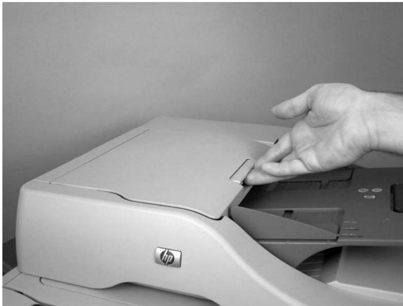
**Figure 5-5** Remove the ADF input tray (1 of 3)
