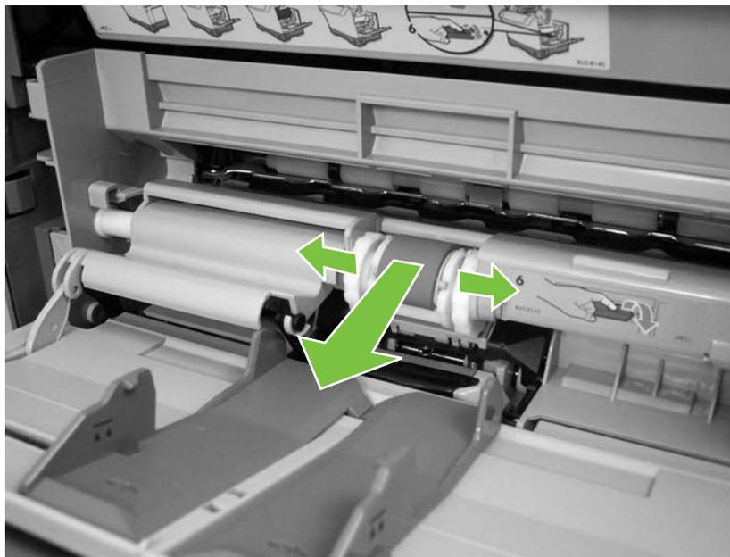
**Figure 5-24** Remove the tray 1 pickup roller
