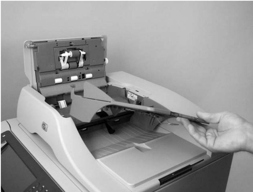
**Figure 5-7** Remove the ADF input tray (3 of 3)
