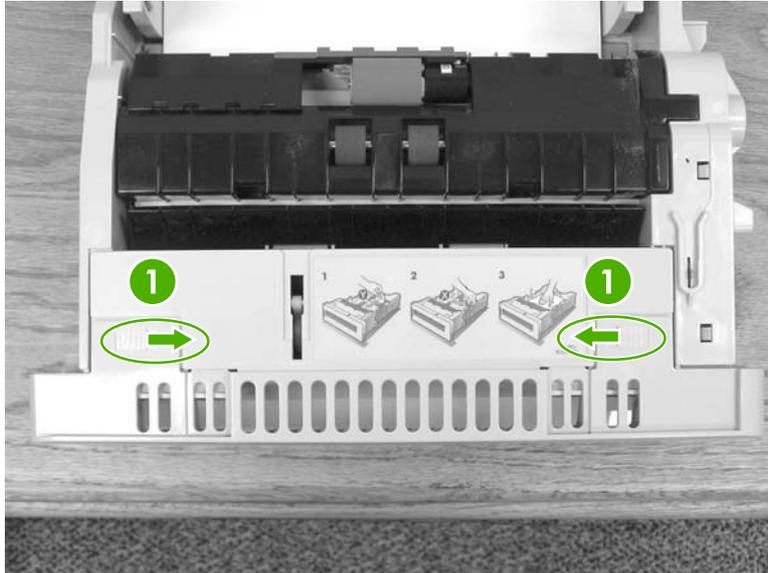
**Figure 6-3** Tray 1 pickup roller and separation pad (1 of 6)
