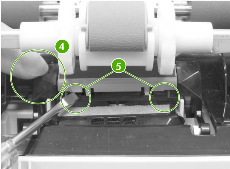
**Figure 6-7** Tray 1 pickup roller and separation pad (5 of 6)
