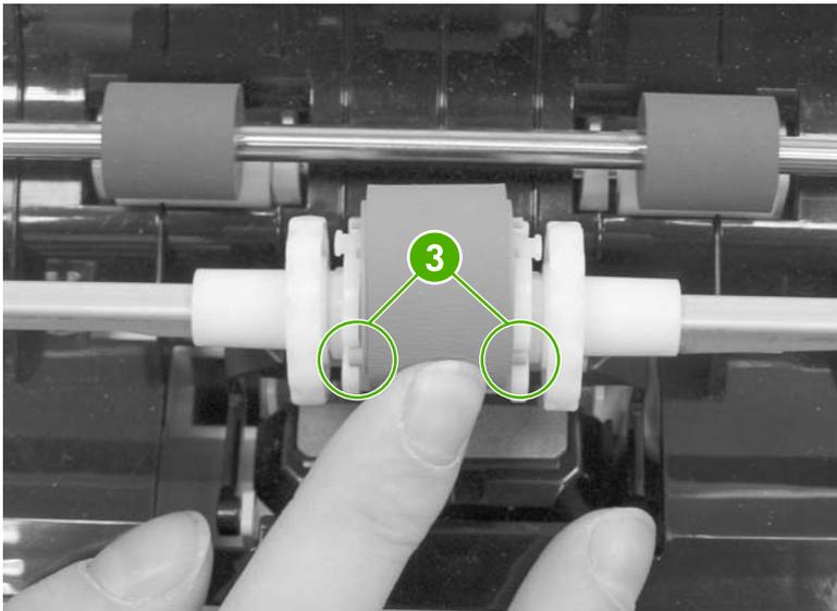
**Figure 6-6** Tray 1 pickup roller and separation pad (4 of 6)
