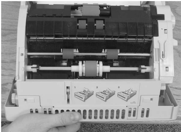
**Figure 6-4** Tray 1 pickup roller and separation pad (2 of 6)
