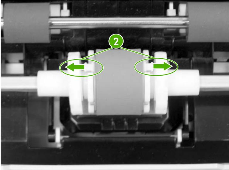
**Figure 6-5** Tray 1 pickup roller and separation pad (3 of 6)
