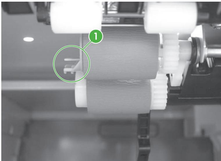
**Figure 6-10** Tray 2-x feed and pickup rollers (1 of 2)
