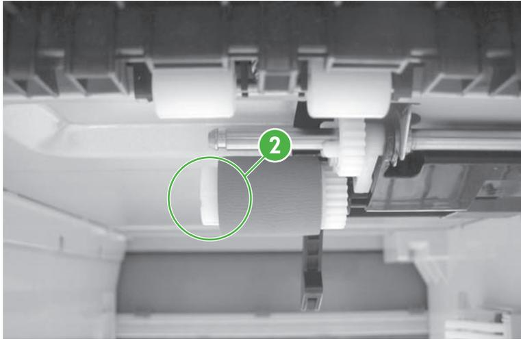
**Figure 6-11** Tray 2-x feed and pickup rollers (2 of 2)
