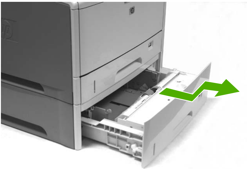
Figure 5-11 Removing the tray 3 retard roller (1 of 2)
