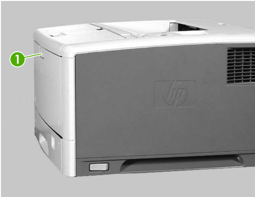
Figure 5-3 Removing the tray 1 pickup roller (1 of 3)
