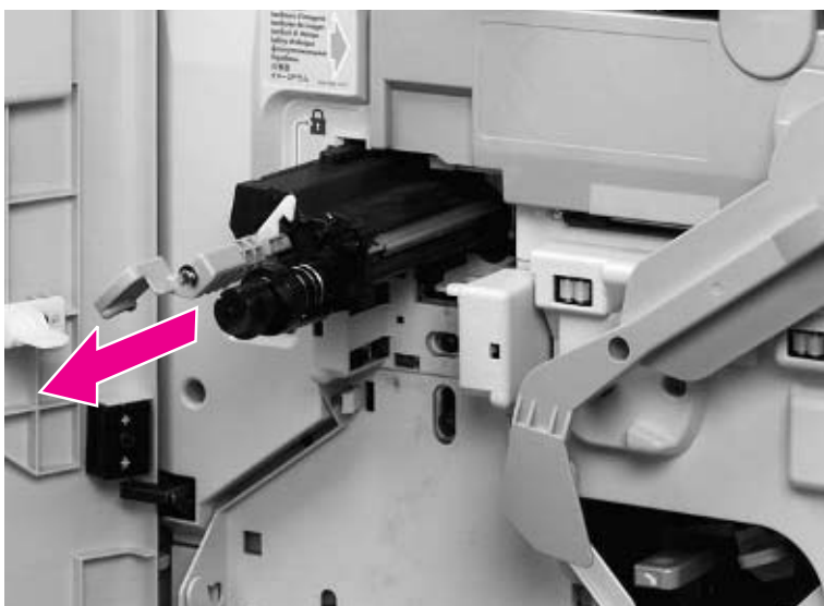
Figure 79. Remove the transfer cleaner
