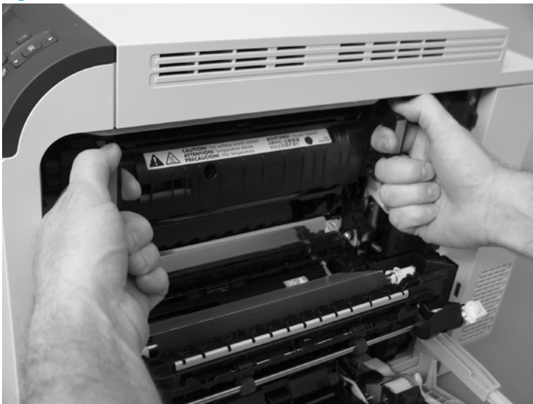
Figure 1-28 Remove the fuser (2 of 2)
