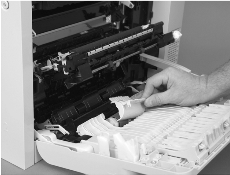
Figure 1-68 Remove the pickup roller (Tray 1; 3 of 5)
