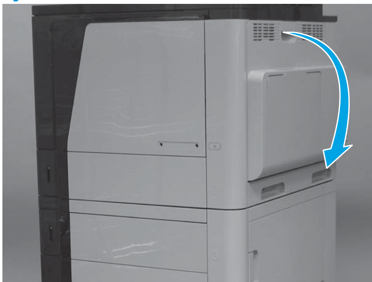
Figure 1-29 Remove the intermediate transfer belt (1 of 4)
