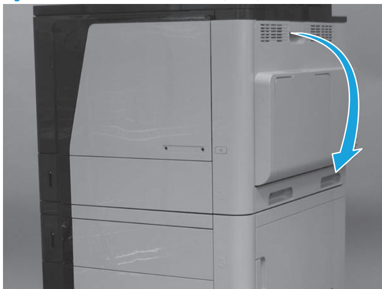
Figure 1-73 Remove the transfer roller (1 of 3)
