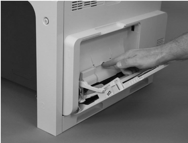
Figure 1-67 Remove the pickup roller (Tray 1; 2 of 5)
