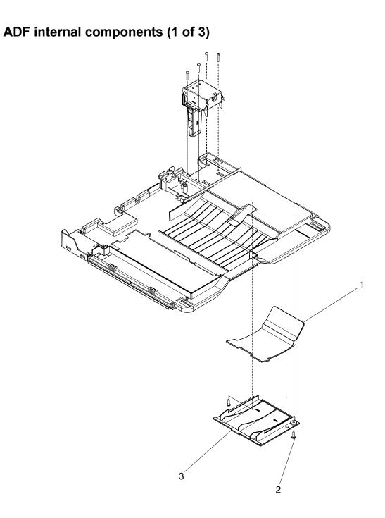
Figure 8-31 ADF internal components (1 of 3)
