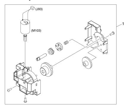
Figure 8-21 Lifter-drive assembly
