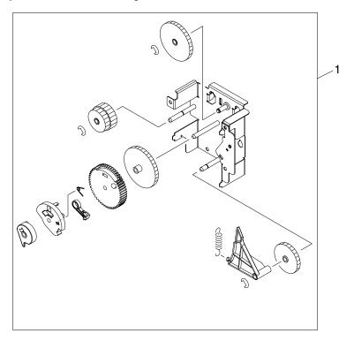
Figure 8-20 Paper-pickup-drive assembly
