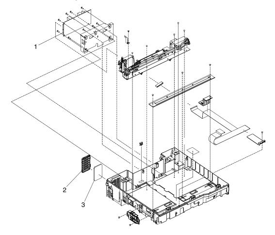
Figure 8-42 Scanner-base components
