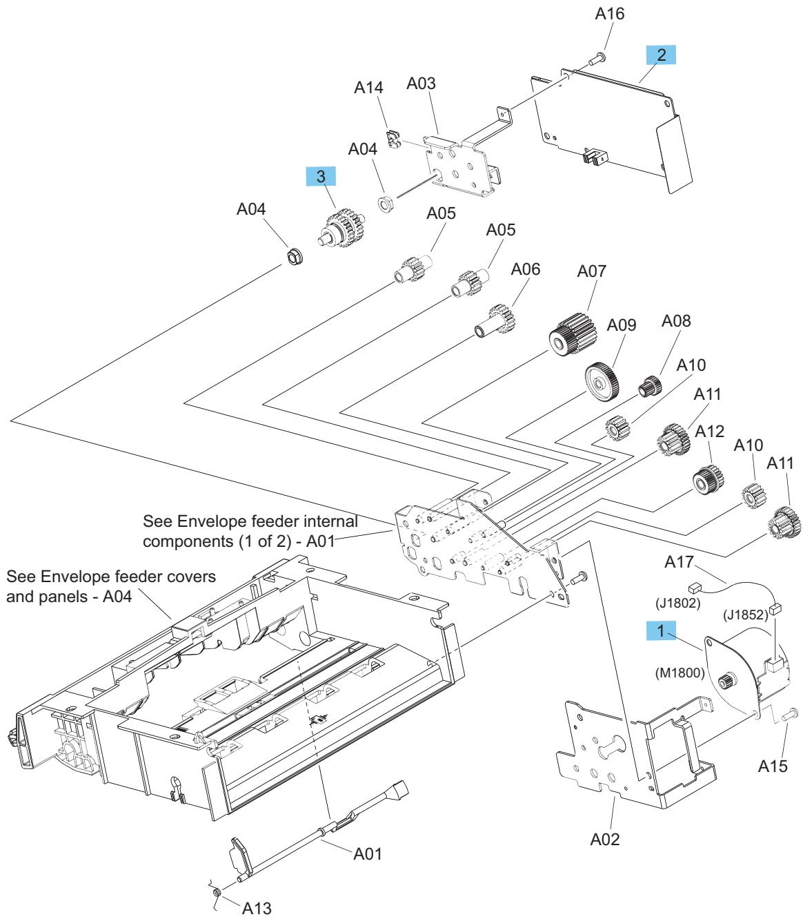
**Table 2-12 Envelope feeder internal components (2 of 2)**
