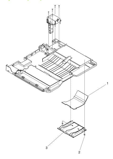
Figure 7-31 ADF internal components (1 of 3)
