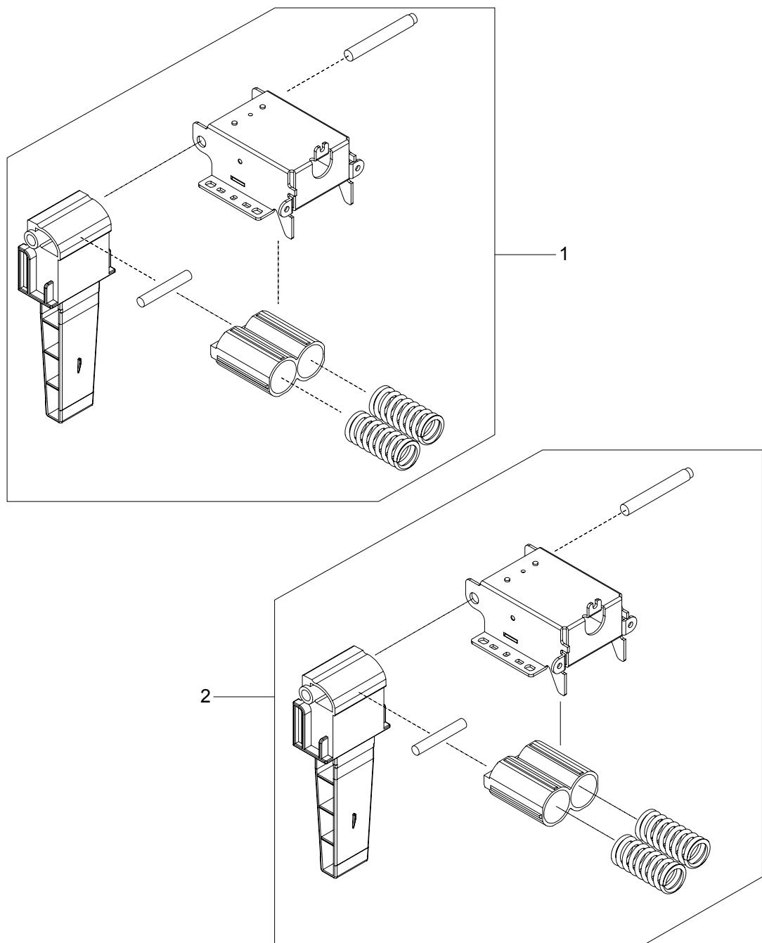
Figure 7-32 ADF internal components (2 of 3)
