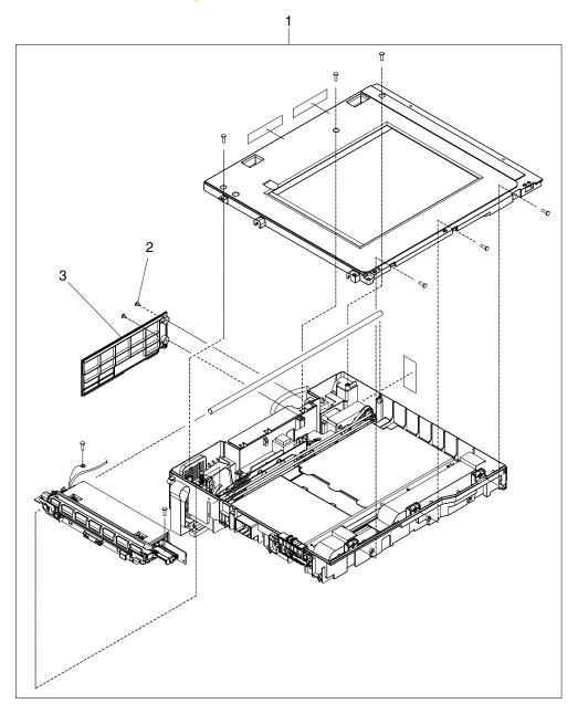
Figure 7-42 Scanner flatbed-unit assembly
