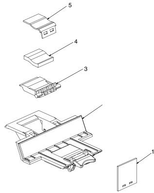
Figure 7-8 Separation pad assembly (ADF)
