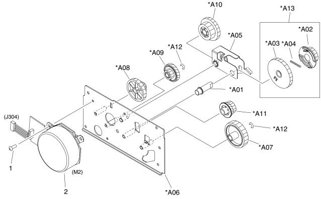
Figure 7-28 Fuser drive assembly (print engine)
