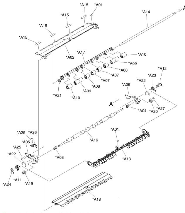
Figure 7-34 Registration assembly (print engine)
