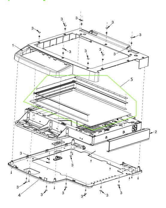
Figure 7-12 Scanner top assembly
