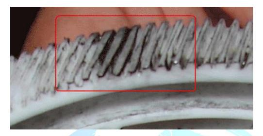
The drum drive assembly (includes: Guide, gear shift A, Guide, gear shift B, Gear 193T, Spring compression, bushing, Side plate drum drive, and Cap drum gear) is set up as a service part, part number RM1-8493-000CN.
