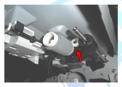
This gear is not available alone however is included on the paper feed shaft assembly RM1-8424 as shown.
