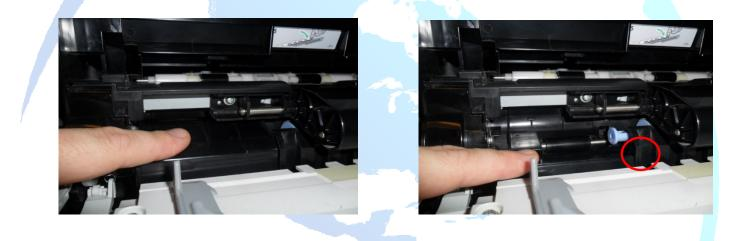
To gain full access to this area, the tray 1 pick up assembly must be completely removed, then check to verify functionality of the feed flag and to see any hidden obstructions.
