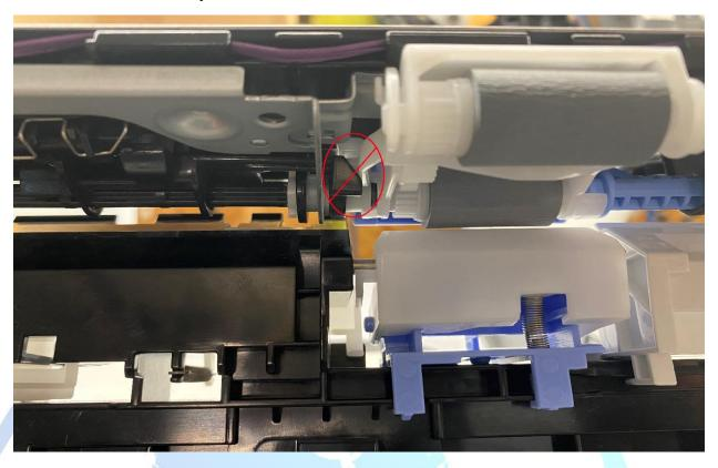
If the left white arm is pushed in, the roller bracket should drop down:
