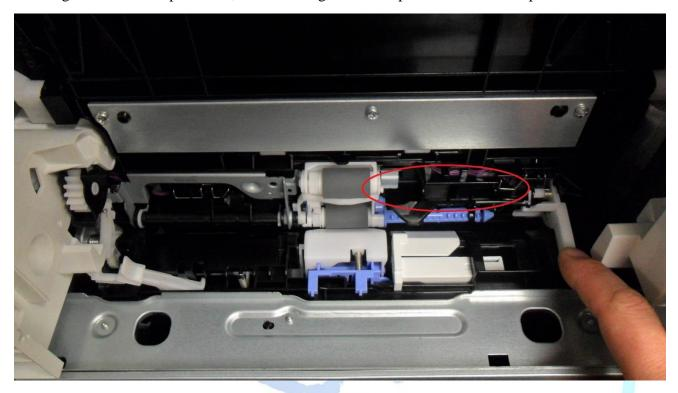
If the paper sensor flag is missing, damaged, or dislodged replace the Paper Pickup Assembly **RM2-6771**.
