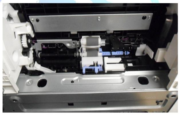
Note the roller's white tab hooks onto the metal pick up arm
