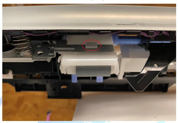
The white roller actuator should lift up the black flag for the printer to recognize the tray has lifted
