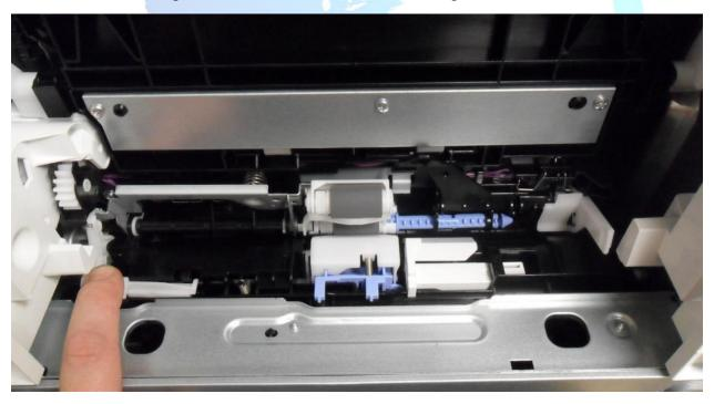
2. Check if the Pickup rollers are worn out.
