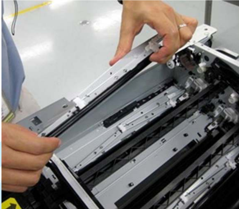
Figure 15: Continue to keep the shutter arm squeezed together as it is removed from the printer
