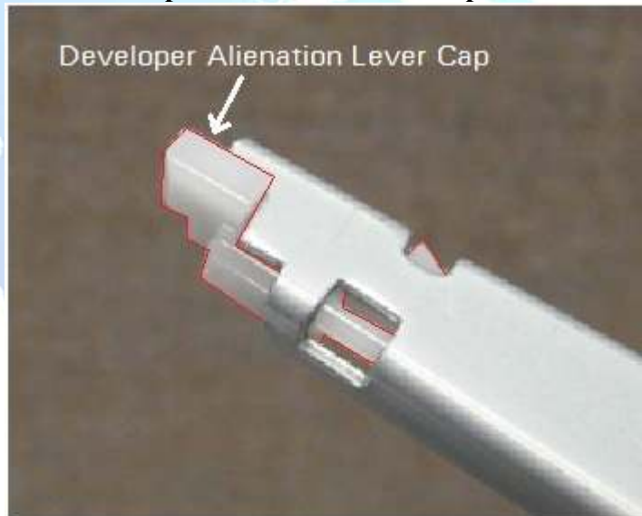
Figure 7: View of the Developer Alienation Lever Cap attached to the end of a shutter arm with the Main Drive Assembly removed
