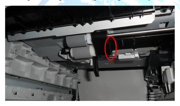
With the printer on its back pull the retaining tab on the black housing forward until it pops back into position allowing the flag on its right side to now trip PS 907. See Figure 2.
