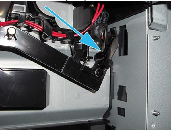
• Notice how the Metal finger is behind the plastic rocker arm
