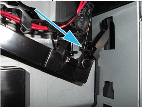
The metal switch finger should be "in Front" of the plastic rock arm.
