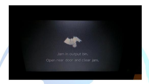
The Jam in output bin message has been a common occurrence for the above listed models. To troubleshoot, closely examine the paper exit area for any obstruction and open the rear door to inspect for obstruction.
