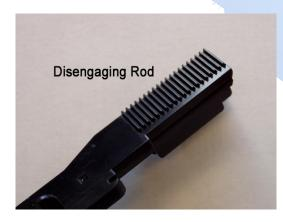
The developing disengaging rod will raise approx. an inch, pause for 2 seconds, and then raise a second time.
