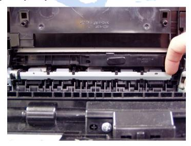
If the issue is confirmed, carefully move the guide to left or right to see if it will go to its home position. If not, a close look will be needed to determine the cause of the problem and may need to contact LPI tech support for further diagnosis.
