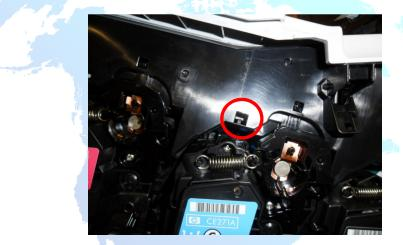
This issue may be addressed by snapping the guide back into position. In order to do this, it is necessary to use a small flat-blade screwdriver and firmly press to help lock the tab behind the sheet metal as shown below. Photo with correct positioning:
