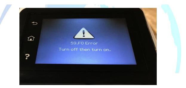
The 59.F0 has been a common error code on the HP CLJ M452 and M377 / M477 MFP models. The printers service manual references this error to a "drum motor assembly" but in most cases has been resolved by replacing the Transfer Belt assembly (RM2-6454). The belts have an internal failure that the prevents the secondary transfer rollers from engaging, and need to be replaced as a whole unit.
