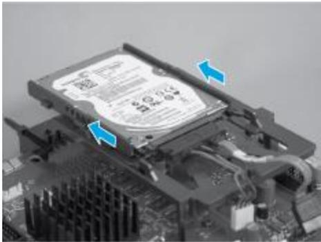
8. Remove the connector assembly from the HDD. (Transfer the connector assembly to the new HDD.)
