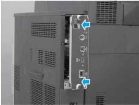
15. Tighten the formatter screws
