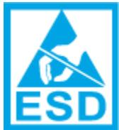
**Electrostatic sensitive device. Always perform service work at an ESD-protected workstation or mat, or use an ESD strap. If an ESD workstation, mat, or strap is not available, ground yourself by touching the sheet-metal chassis before touching an ESD-sensitive part.**
