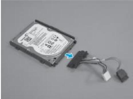
9. Remove the new HDD and rails from the packaging. Recycle the used HDD according to local regulations.
