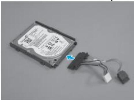
12. Slide the HDD into the bracket.
