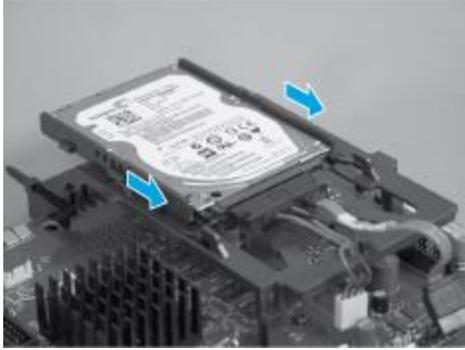
13. Connect the two HDD connectors to the formatter.
