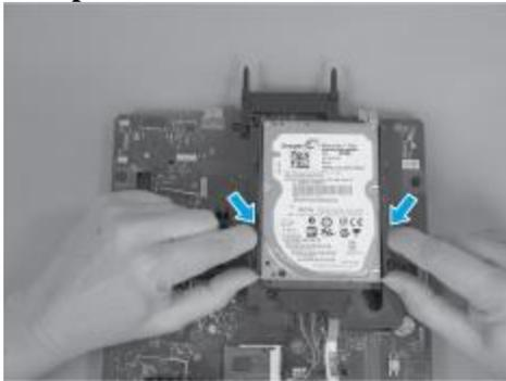
7. Slide the HDD in the direction of the arrow to remove it from the bracket.
