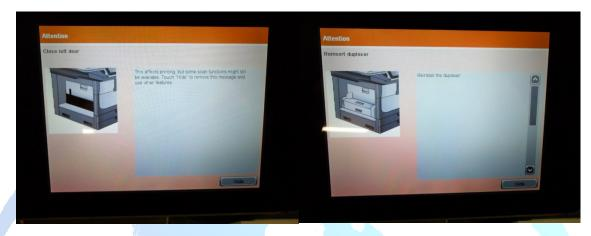
There have been a few cases where the printer will display one of the above messages without the ability to print. The cause of this has been the rear fuser lock tab being just out of the locked position, which will intern cause the linkage to the switch "SW1 fuser/left door" incomplete.
