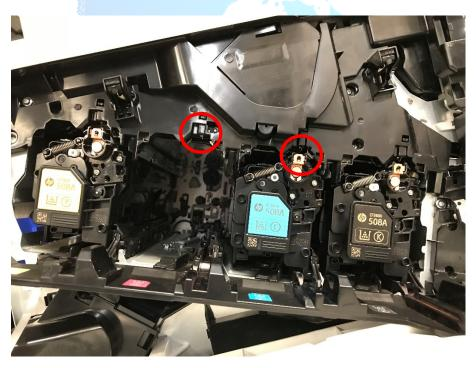
This issue may be addressed by snapping the guide back into position. In order to do this, it may be necessary to remove screws and use a small flat-blade screwdriver and firmly press to lock the guide to the sheet metal frame.
