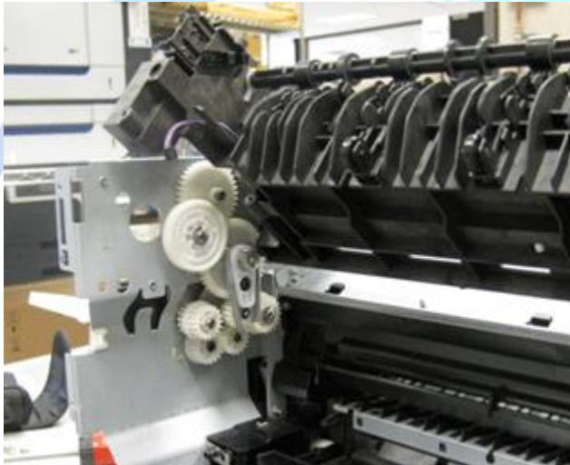
Figure 2: Releasing the output roller assembly
