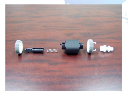
The RM1-0731 and RM1-6313 roller are complete assemblies that just snap in the printer. The difference on the rubber coated idler rollers vs. plastic idler rollers (on the outside of the main roller hub) has not affected print performance on any model.
