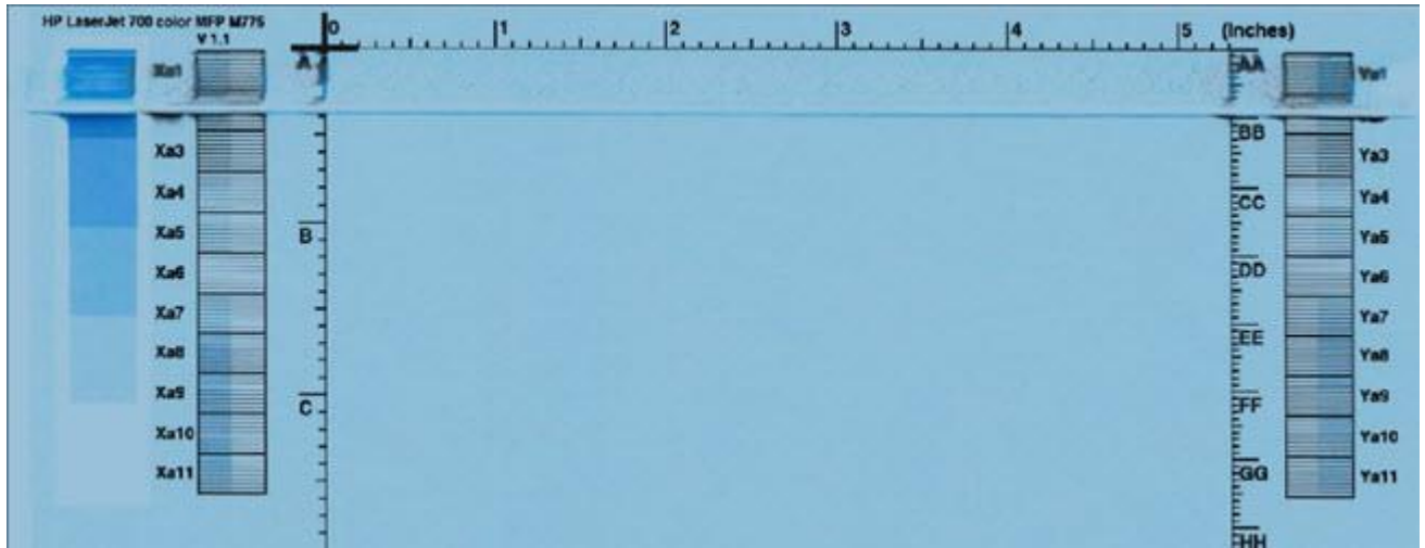
Figure: The Mylar strip needs to be cleaned and/or is damaged (PQ defect at the top of the page)
