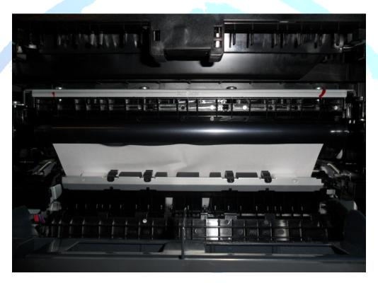
The cause for this paper jam is that the transfer belt is *not* rotating within the printer.
