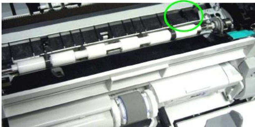
Figure 1: Paper width sensors (PS106 and PS112)
