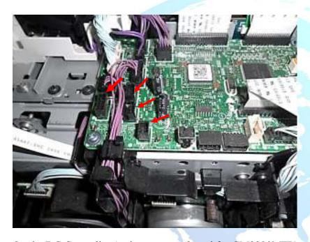
On the DC Controller (or interconnect board for CM2320MFP), unplug the cables from connectors: J162, J163, J164, J165, J166, and J155
