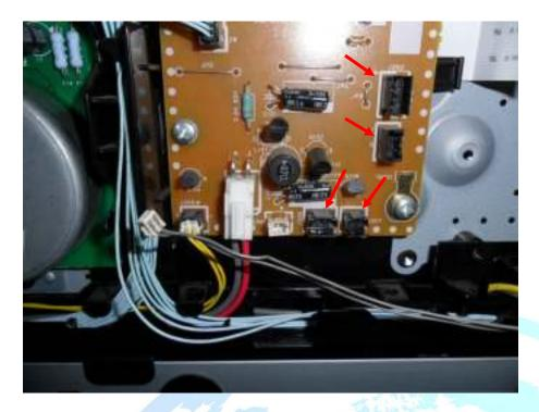
Unplug the cables on the Driver PCA from connectors J202, J203, J206, and J207
