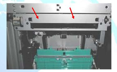
Remove 2 screws, and Pickup Assembly by lifting up on metal plate.
