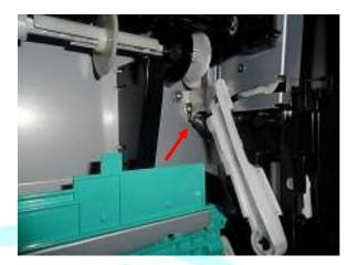
Unhook the spring from the lift arm and the frame on both sides
