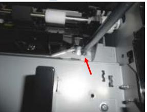
Remove 2 screws on the registration to remove registration
