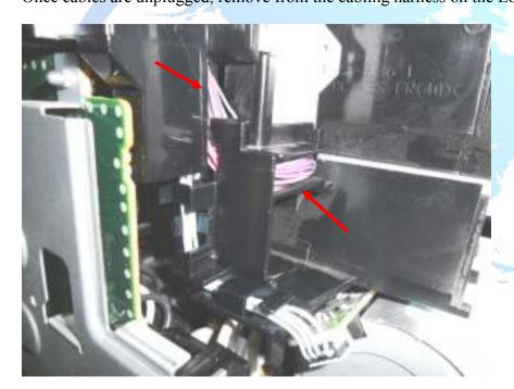
Remove the cables from the cable harness
