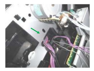
Release the tab {Blue arrow} Slide cable guide out to back of printer
