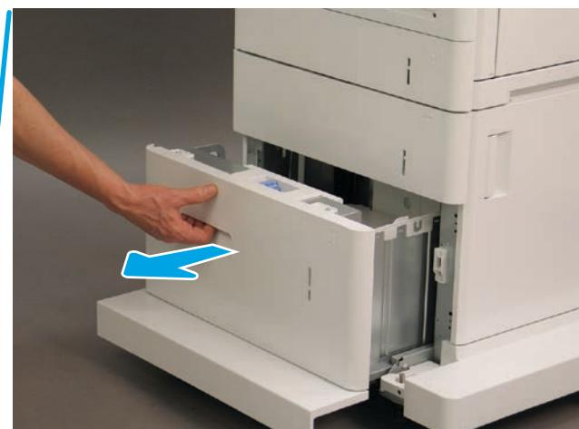
**EN** Open the paper tray for which the rollers will be replaced.
