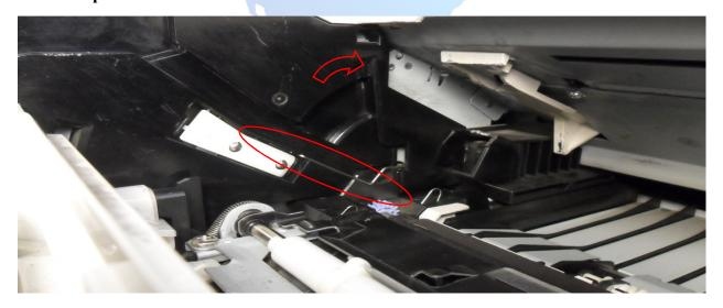
If found in the incorrect position, it can be manually placed back into its retaining groove
