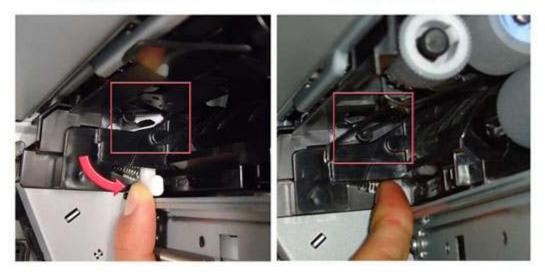
3.Install the tray cassette and check if the level indicator moves while the tray mechanism is lifting.
