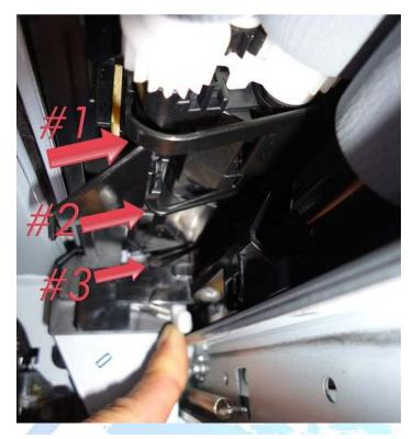
2.Remove any piece of paper found in the tray-closed tab area. Manually push the white tab towards the right to lower the sensor flag down, this will allow you to see underneath the rear side of the media stack sensor. Push the white tab several times, the sensor flag can occasionally get stuck and this movement will help to release it.
