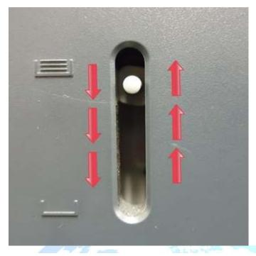
4.Perform a manual sensor test and check the paper surface sensor (letter Q). The idle value for this sensor is "1" when the tray is filled with paper and closed. Ensure the default value changes when manually moving sensor.
