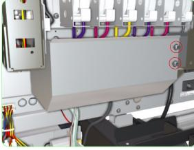
**14.** Remove two screws that secure the metal cover to the front of the Printer.
