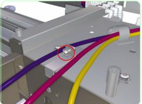
**17.** Remove the screw that is used to secure the spring.
