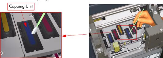
Make sure that the Cap Cleaning Liquid does not drip on to other parts of the Printer. If the Cap Cleaning Liquid drips on to the Belt or any nearby Sensors, this could cause serious damage to the Printer.
