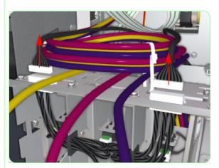
**5.** Cut the cable tie that secures the Ink Tubes.
