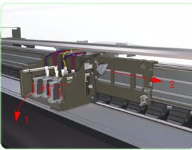
20. Remove the three screws that you loosened in step 15, and then move the headbase slightly toward the paper-output side of the printer so that you can then slide the carriage base toward the wiping side.
