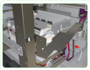
**11.** Remove the Gear Cover from the Wiping Station.
