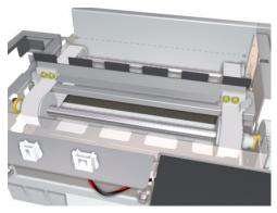
2 Tighten or loosen the Tension screw on both sides of the Wiping Station (for each Wiper Belt) until the remaining length of the screw is 13 mm.
