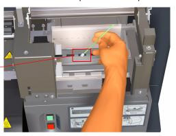
Make sure that the Wiper Cleaning Liquid does not drip on to other parts of the Printer. If the Wiper Cleaning Liquid drips on to the Belt or any nearby Sensors, this could cause serious damage to the Printer.
