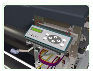
**6.** Remove two screws that secure the Front Panel to the Printer.
