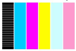
In this situation it is recommended to perform the Printhead Recovery procedure  $\Rightarrow$  Refer to the User's Guide.
