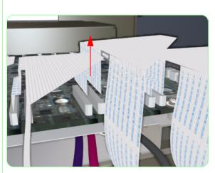
**6.** Remove two screws that secure the Printhead Connector Assembly to the Printhead.
