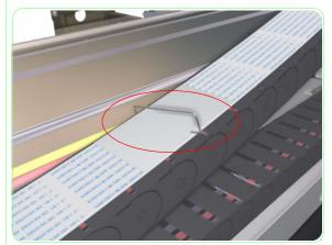
**51.** Attach the three metal clips to secure the cables to the cable carrier.
