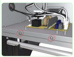
**7.** Remove two screws that secure the Heater Relay Assembly to the Printer.
