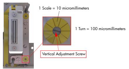
5 If for example, the deviation measured in step 2 was 240 micro-millimeters, you would turn the Vertical Adjustment Screw 2 full turns and 4 scales.
