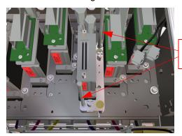
Printhead Positioning Pins
