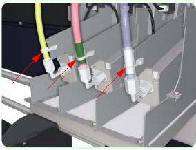
**29.** Cut the Insulock ties (but do not loosen the plastic nuts) and drain the ink from the subtank. When the flow of ink stops, pull the tube through from the back to the front side and drain the rest of the ink from the subtanks.
