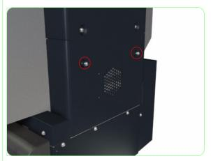
**1.** Remove two screws that secure the Lower Side Cover to the Printer.
