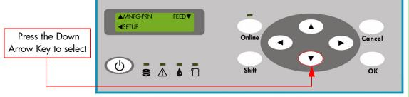
2 During the manual feed process, the following message will appear on the Front Panel:
