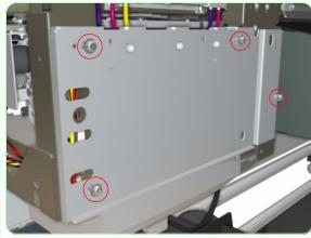
**9.** Remove four screws that secure the metal plate to the chassis.
