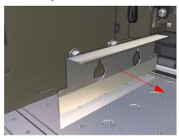
3 Make sure that the Printhead Height Lever is in the **upper** position (so that the Printhead height is actually in the **lower** position). Make sure you loosen the two Printhead Height Adjustment screws before trying to change the position of the Printhead Height Lever and make sure you tighten the screws after changing the Printhead Height.
