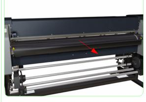
2. Pull out the Front Heater slightly.
