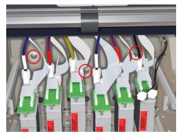
To loosen the three screws, you will need a 3mm Allen Key that is at least 20 cm long.
