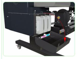
**3.** Open the Ink Cartridge Door and remove from the Printer.
