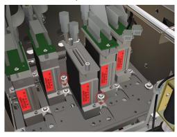
2 Install the Printhead Adjustment Jig 1 in to position against the Carriage Base Plate. Make sure that the 2 datum pins touch the Printhead as shown.
