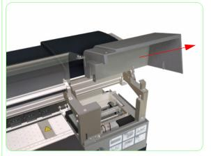
**3.** Slide the Wiping Door to the right and remove from the Printer.
