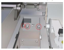
7 Adjust the Wiping Station so that it is level with the aluminum frame piece on the left rear of the Wiping Station. Make sure that the Wiping Station is as level as possible before tightening the screws in the next step.
