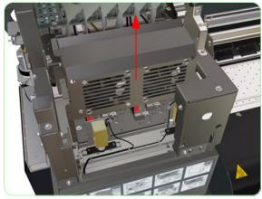
**10.** Remove the Printhead Cooling Fan Assembly from the Printer.
