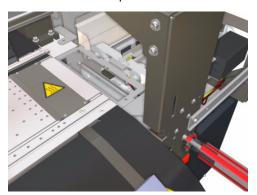
Make sure that the Carriage is Uncapped before performing the following step. Trying to move the Carriage out of the Capping Station while it is still capped will cause damage to the Printheads.
