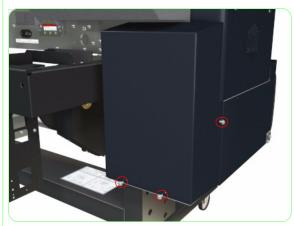
**1.** Remove three screws that secure the Rear Ink Cartridge Cover to the Printer.
