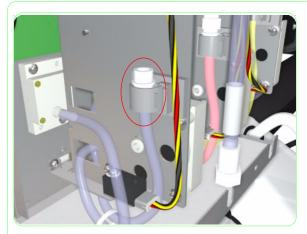
**TIP**: It is helpful to clip the lower part of the tube to the plastic securing clamp to keep it in an upright position while draining the top part of the tube.
