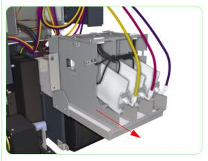
**8.** Carefully pull out the Subtank Station slightly.
