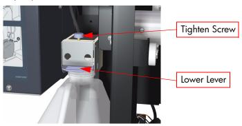
**6** Once the Waste Ink Bottle is correctly installed, the Front Panel will request you to reset the Waste Counter.
