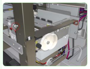
**10.** Remove two screws that secure the Gear Cover to the Wiping Station.
