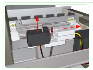
**19.** Disconnect the Sensor Cable from the Right Rear Cover Sensor and remove from the Printer.
