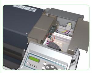
**4.** Remove two screws that secure the Home Position Sensor to the Printer.
