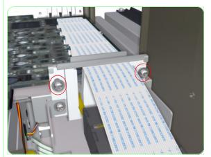
**12.** Remove two screws that secure the metal bracket to the Carriage Assembly.
