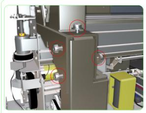
**19.** Remove four screws that secure the Left Capping Frame at the top.
