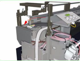
**20.** Disconnect the cable carrier and lay it flat, out toward the side of the printer.
