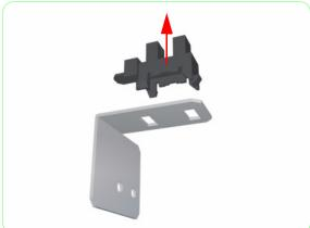
**7.** Unclip the Home Position Sensor from the Support Bracket.
