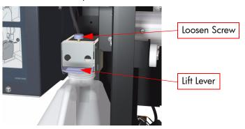
**2** Carefully pull out the Waste Ink Bottle, taking care not to spill any on the Printer or on the floor.
