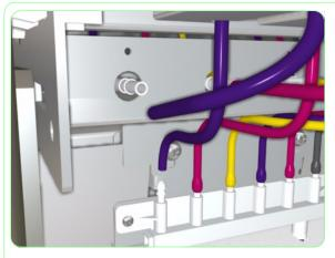
**14.** Disconnect the Priming Tube from both ends.
