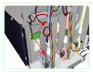
**26.** Detach each tube from its plastic securing clamp.
