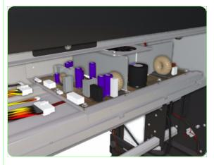
**4.** Disconnect ALL the cables from the Power Supply Unit.
