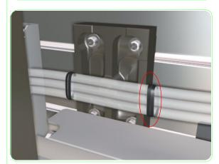
**47.** Secure the tubes with the twist-ties and clamps.
