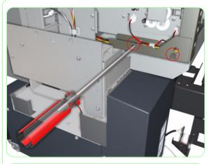
**11.** Remove two screws that secure the metal cover to the side of the Printer.
