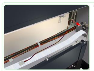
**5.** Remove the Front Media Sensor from the Printer
