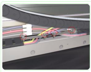
**16.** Remove the two screws from each of the tube-holder brackets.
