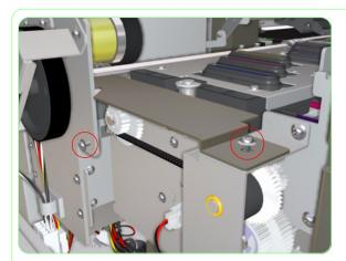
**16.** Remove two screws that secure the metal bracket to the Capping Station.
