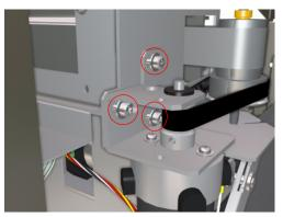
3 Hook the Push/Pull Gauge onto the Scan-Axis Motor Bracket and tension the Scan-Axis Belt to a force of 41.0 N  $\pm$ 2.0 N (4.18 kgf  $\pm$ 0.2 kgf).
