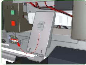
**9.** Remove the metal bracket from the Wiping Station.
