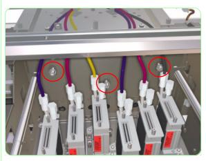
**15.** Loosen the three screws that are used to secure the carriage to the headbase. You will remove them in a later step.
