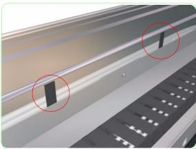
**41.** Secure the tubes to the back rail using the bendable tabs.
