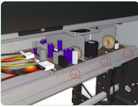
**3.** Remove three screws that secure the Power Supply Unit to the Printer from the front.
