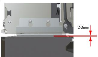
**4** While holding the Carriage Shield in position, tighten the two screws that you loosened in a previous step.
