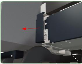
**5.** Remove two screws that secure the Left Subtank Cover to the Printer.
