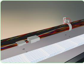
**3.** Remove one screw that secure the Cable Holder to the Printer.
