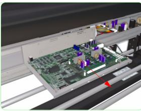
**6.** Remove the Main PCA Tray from the Printer.
