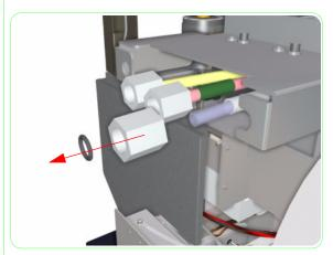
**21.** Remove the plastic nut from the tips of the three tubes on both sides of the cable carrier. If the nuts are difficult to remove, you can cut the tubes.
