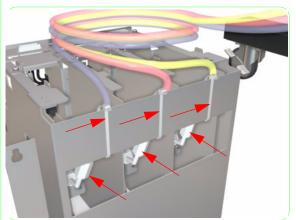
**38.** Cut the Insulock ties, loosen the plastic nuts, and remove the supply tubes.
