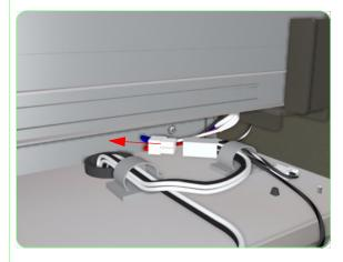
**4.** Disconnect the Heater Relay Cable.
