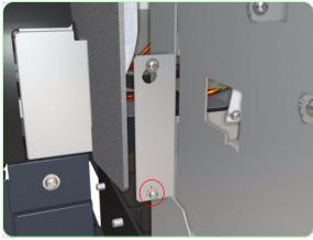
**7.** Remove one screw from each side of the Subtank Station.
