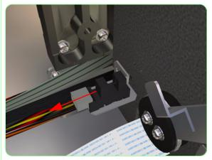
**4.** Remove the Media Lever Sensor from the Printer.
