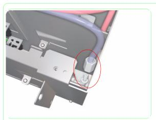
**39.** Disconnect the supply tubes from the subtank and dispose them according to local regulations.
