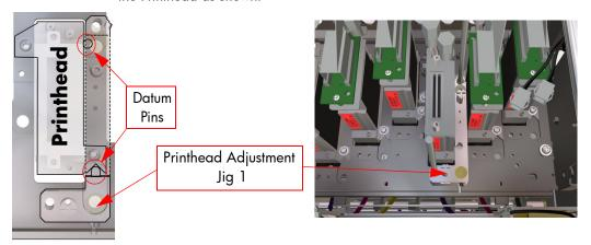
7 Install the two screws to secure the Printhead. The screws should not be tightened too much, just enough so that the Printhead does not move loosely.
