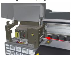
4 Using the Push/Pull Gauge, measure the tension in the middle of the Carriage Belt. The tension measured should be between 120 and 140 g.
