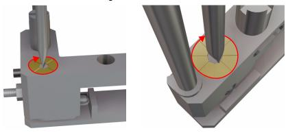
**6** Once the Printhead Adjustment Jig 1 has been calibrated, you can loosen the fixing screws, remove the Printhead Positioning Pins and remove the Printhead Adjustment Reference Plate.
