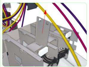
**11.** Remove the Sensor Plate from the Subtank Station.
