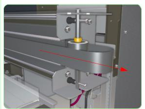
**10.** Carefully slide the Belt out of the Carriage Assembly and remove from the Printer.
