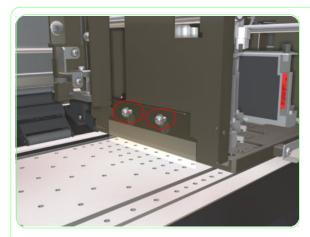
**13.** Remove the two screws that are used to secure the plate assembly.
