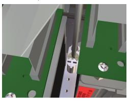
12 Tighten the front screw that secures the Printhead to the Carriage Base Plate.
