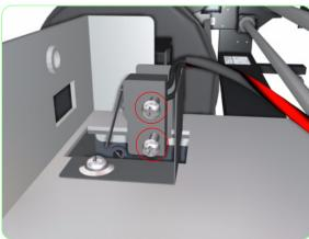
**6.** Remove two screws that secure the IC Door Sensor to the Ink Supply Station.
