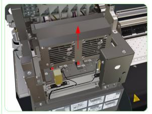
**8.** Raise the Printhead Cooling Fan Assembly slightly.
