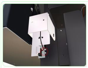
**7.** Remove two screws that secure the Waste Bottle Sensor to the Bracket.
