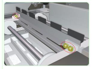
**3.** Remove four screws that secure the Wiper Blade to the Wiper Belts.
