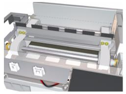
**3** Remove the Carriage Shields from both sides of the Carriage Assembly.
