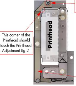
Make sure the Printhead Adjustment Jig 2 is located against this pin
