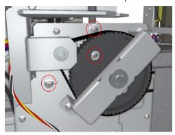
**3** Hook the Push/Pull Gauge onto the Paper-Axis Motor Bracket and tension the Paper-Axis Belt to a force of 49.0 N  $\pm$ 2.0 N (5.0 kgf  $\pm$ 0.2 kgf).
