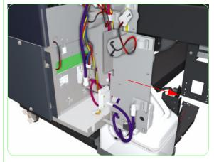
**8.** Remove the Ink Pump Assembly from the Printer.
