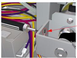
Hook the Push/Pull Gauge onto this hole
