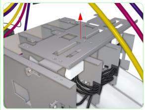
**10.** Remove the metal plate from the Subtank Station
