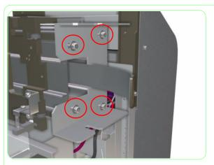
**25.** Remove the four screws that are used to secure the bracket to the printer body.
