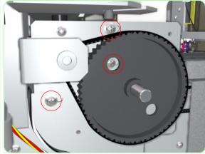
**7.** Loosen three screws that secure the Paper-Axis Motor Bracket to the Chassis.
