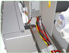
**20.** Remove two screws that secure the Left Capping Frame to the bottom.
