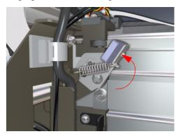
**3** Loosen five screws from the left hand side of the Capping Station.
