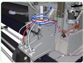
**57.** Feed the disconnected end of the subtank tube to the supply-pump side of the printer.
