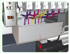
**13.** Pull the metal cover down slightly so that the Priming Tubes are exposed.
