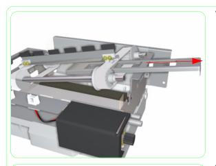
**12.** Remove the metal plate from the Wiping Station.
