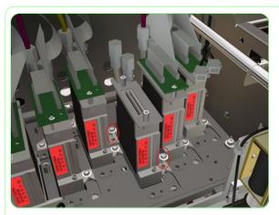
**10.** Remove two screws that secure the Printhead to the Carriage Assembly.
