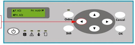
1 In the Printhead Adjustment submenu, scroll to "PH Adj Print" and press the OK key.
