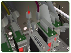
9. Install a Tube Cap on to the Printhead.
