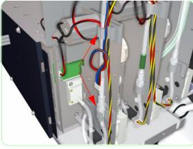
**59.** Clip the tube into the plastic securing clamp.
