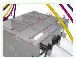
**9.** Remove eight screws that secure the metal plate to the Subtank Station.
