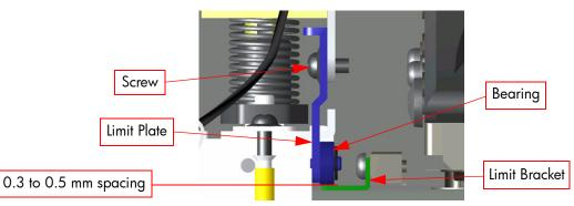
6 Tighten the screws that secure the Plates.
