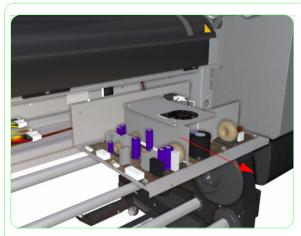
**5.** Remove the Power Supply Unit (including the Support Tray) from the Printer.
