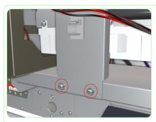
**8.** Remove two screws that secure the metal bracket to the Wiping Station.
