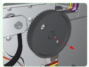
**8.** Release the Belt and remove the Paper-Axis Gear from the Printer.
