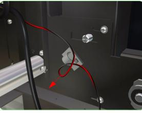
**2.** Release the End-of-Media Sensor Cable from the Cable Holder.
