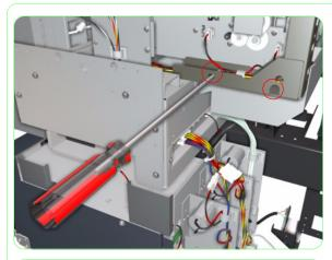
**13.** Remove two screws that secure the metal cover to the side of the Printer.
