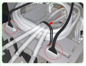
**60.** Connect the cables to the subtank and ensure that the tubes are secured with a twist-tie as shown in the image.
