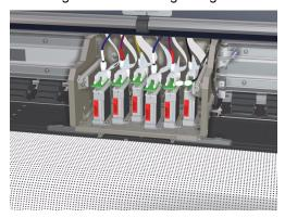
6 Lift the Carriage slightly and reposition the Carriage Height Tools. The front Tools should be positioned so that the Carriage is sitting on top of step C of the tool.
