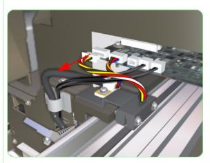
**6.** Remove two screws that secure the Encoder Sensor.
