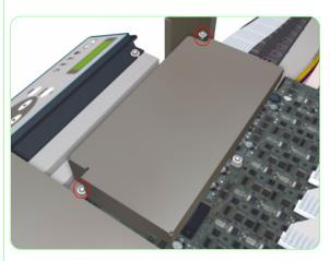
**6.** Remove the Carriage PCA Cover from the Carriage Assembly.
