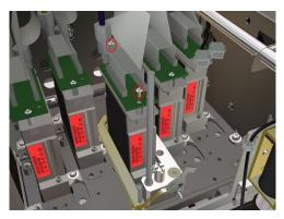
**12** Before moving to the next stage of the Printhead Adjustment procedure, make sure that the Printhead Connector cables are safely secured with tape so that they don't hit other parts of the Printer.
