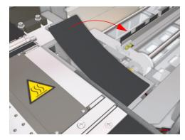
**6** Loosen three screws that secure the Wiping Station on the left hand side.
