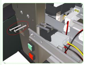
**18.** Remove two screws that secure the Left Rear Cover Sensor to the Chassis.
