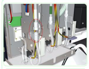
**58.** Connect the subtank tube to the supply pump.
