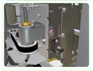
5. Remove one screw that secures the Belt to the left side of the Carriage Assembly and then release the Belt from the Carriage Assembly.
