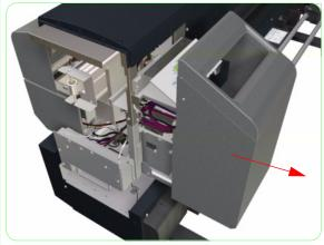
**7.** Remove the Left Subtank Cover from the Printer
