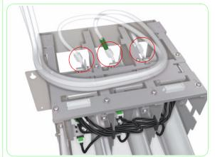
**52.** Connect the tubes on the capping side of the printer to the *back* side of the subtank.
