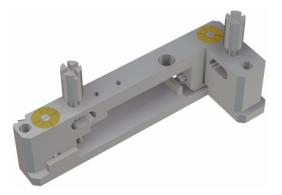
3 Insert the two Printhead Positioning Pins in to the Printhead Adjustment Jig 1.
