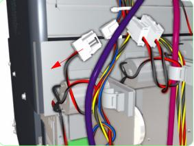
**4.** Disconnect the Ink Pump Assembly cable.
