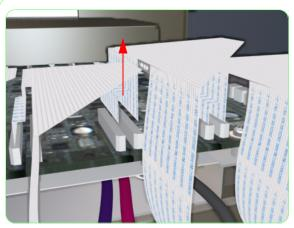
**10.** Disconnect ALL the Printhead Connector Cables from the Carriage PCA.
