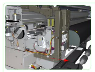
**22.** Remove the Left Capping Frame from the Printer.
