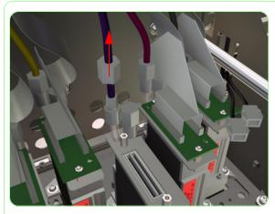
7. Disconnect the Ink Tube from the Printhead.
