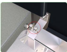
**2.** Remove two screws that secure the Rear Cover to the left hinge.
