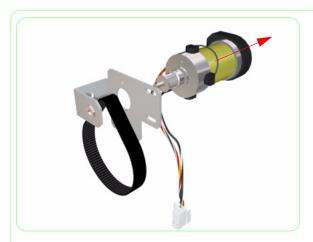
**12.** Remove the Paper-Axis Motor from the Bracket.
