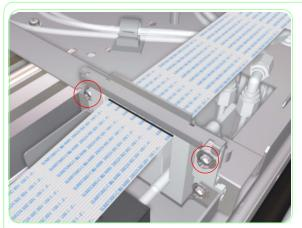
**50.** Use two screws to attach the cable brace to the carriage board.
