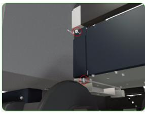
**4.** Remove the Left Electronics Module Side Trim from the Printer.
