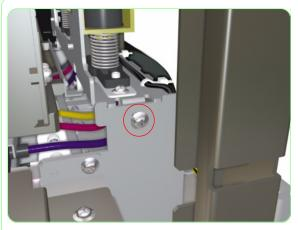
**10.** Remove one screw from each side of the Solenoid Assembly.
