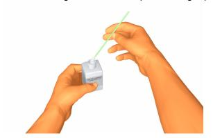
Make sure that you use the Wiping Cleaning Liquid and NOT the Cap Cleaning Liquid to clean the Wiper Blade. The Cap Cleaning Liquid is not strong enough to clean the Wiper Blade properly and could cause damage to the Printheads.
