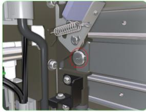
**9.** Remove one screw that secures the Belt to the right side of the Carriage Assembly.
