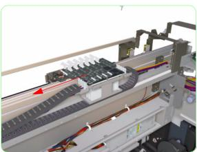
**18.** Uncap the Carriage Assembly and move it out of the Capping Station.
