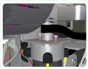
**9.** Remove two screws that secure the Scan-Axis Motor to the Bracket.
