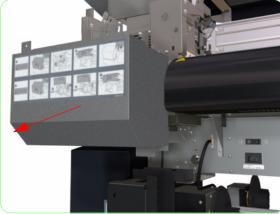
**6.** Remove the Lower Capping Cover from the Printer
