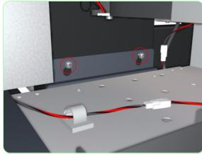
**7.** Loosen two screw that secure the Ink Supply Station to the Printer.
