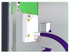
**6.** Remove the two screws that are used to secure the Needle.
