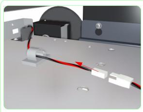
**5.** Disconnect the IC Door Sensor cable.
