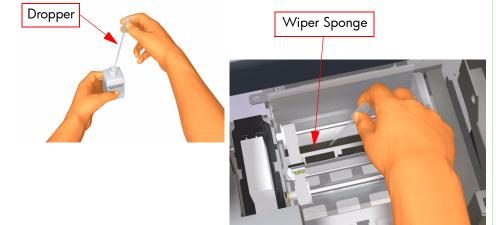
Make sure that the Wiper Cleaning Liquid does not drip on to other parts of the Printer. If the Wiper Cleaning Liquid drips on to the Belt or any nearby Sensors, this could cause serious damage to the Printer.
