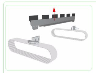
15. Remove the Wiper Blade from the Wiper Belts
