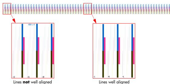
3 In the Printhead Adjustment submenu, scroll to "PH Row Val" and press the ▶ key.
