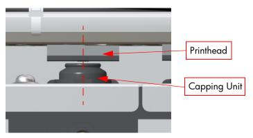
6 If the center of the Capping Units are not aligned with the center of the Printheads, you will need to visually estimate the deviation between the Capping Units and the Printheads.
