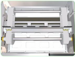
**2.** Manually turn the Wiper Gear so that the Wiper Blade moves to upper position.
