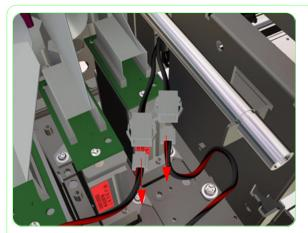
**9.** Disconnect the cables from the Printhead Cooling Fan Assembly.
