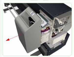
**7.** Remove the Right Subtank Cover from the Printer
