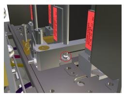
7 Reprint the Check Printhead pattern and measure again the deviation of the Printhead in the vertical position. If there is still deviation, repeat the instructions from step 3.
