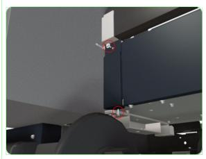
**1.** Remove two screws that secure the Left Electronics Module Side Trim to the Printer.
