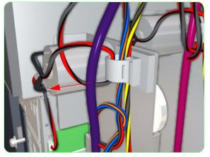
**5.** Remove the Ink Pump Tubes (for ALL three colors) from the cable clip.
