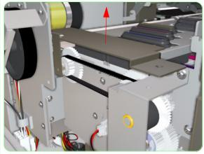
**17.** Remove the metal bracket from the Capping Station.
