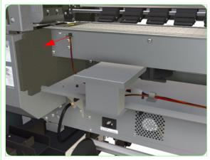
**4.** Remove the Rear Media Sensor from the Printer.
