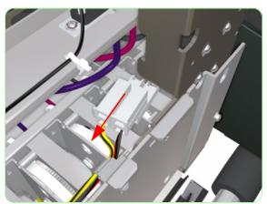
**12.** Disconnect the Cable from the Right Rear Cover Sensor.
