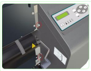
**5.** Remove two screws that secure the Right Subtank Cover to the Printer.
