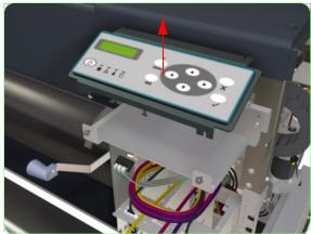
**7.** Remove the Front Panel from the Printer.
