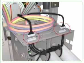
**35.** Remove the electric cable connectors on the subtank.
