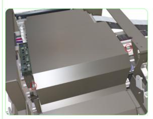
**9.** Remove the Carriage Cover from the Carriage Assembly.
