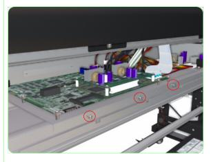
**4.** Remove three screws that secure the Main PCA Tray to the front of the Printer.
