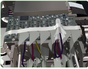
**8.** Cover the Ink Tube carefully with a paper cloth and secure it to the Carriage Assembly with some tape.
