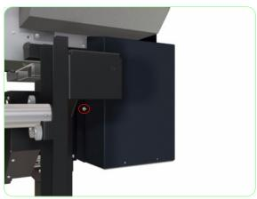
**2.** Loosen one screw that secures the Rear Ink Cartridge Cover to the Printer.
