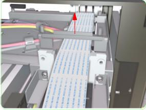
**14.** Remove the cable bracket.
