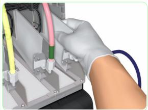
**31.** Press and flatten the subtanks to remove as much ink as possible. This is the best way to ensure against creating an inky mess on and around the printer.
