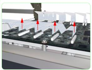
**9.** Disconnect the Trailing Cable from the Carriage PCA.
