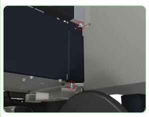
**3.** Remove two screws that secure the Right Electronics Module Side Trim to the Printer.
