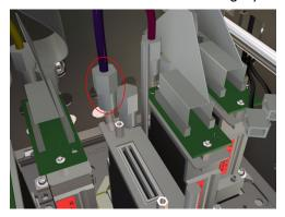
**11** Attach the Printhead Connector Assembly to the Printhead and secure it with 2 screws.
