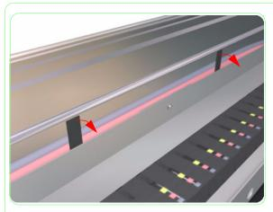
**23.** Bend out the tabs that are used to secure the ink-supply tubes.
