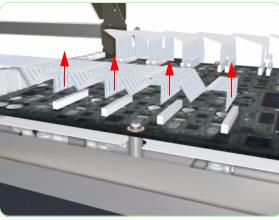
**14.** Disconnect the Trailing Cable from the Carriage PCA.
