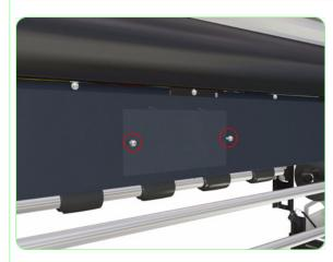
**1.** Remove two screws that secure the Firmware Access Cover to the Printer.
