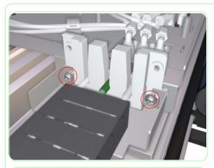
**48.** Use four screws to attach the two cable holder plates.
