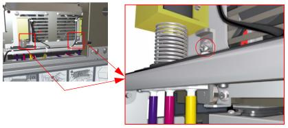
5 Lower each Limit Plate until the bearing (attached to the Plate) almost touches the Limit Brackets on the Capping Station. The space between the Bearing and the Limit Brackets should be between 0.3 and 0.5 mm.
