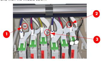
Before tightening the screws, make sure you place some weight (using your finger) on the front of the Carriage. If this is NOT done, the Carriage will be incorrectly adjusted and could cause some serious Print Quality issues.
