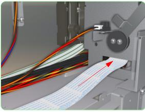
**17.** Pass the Trailing Cable through the hole (as shown in the drawing).
