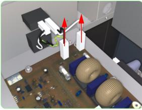
**6.** Disconnect the cables from the power switch.
