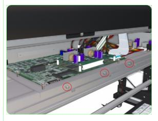
**4.** Remove three screws that secure the Main PCA Tray to the Printer from the front.
