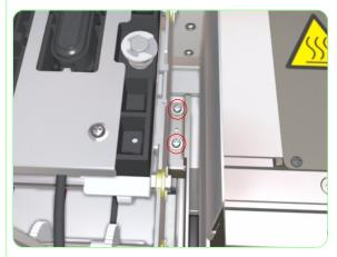
**24.** Remove two screws that secure the Right Capping Frame to the bottom.
