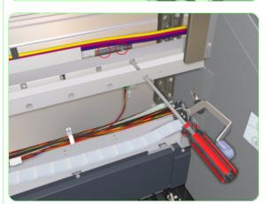
**14.** Remove two/three screws that secure the Pinchwheel Bracket (that secures the Pinchwheel Assembly that you want to remove).
