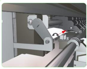
**9.** Remove the C ring that secures the Linkage to the Pinchwheel Cam.
