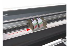
3 Insert the Carriage Height Adjustment Tool (with hole) under the Carriage at positions 3 and 4 as shown below.
