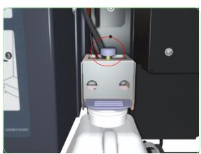
**25.** Loosen the screw that locks the Waste Bottle Bracket into place. You will use the waste bottle to collect the ink.
