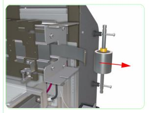
**24.** Release the Belt and remove the Drive Pulley from the printer.
