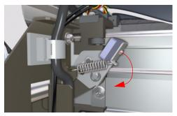
4 Loosen the screw which secures each Capping Limit Plate to the Carriage.
