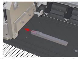
9 Once the Tool stops going in, make sure that it has reached the correct measuring point by moving it in the directions shown until it hits the right and left walls. Once in the correct position, check the Carriage height.
