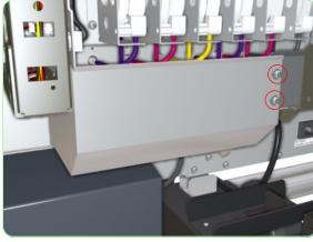
**12.** Remove two screws that secure the metal cover to the front of the Printer.
