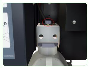
**1.** Loosen the screw that locks the Waste Bottle Bracket into place.
