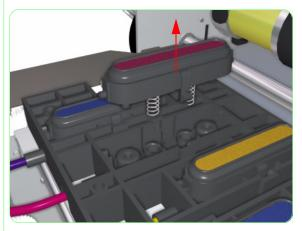
**5.** Release the Capping Unit and remove from the Capping Station.
