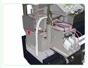
**15.** Lay the cables flat over the side of the printer.
