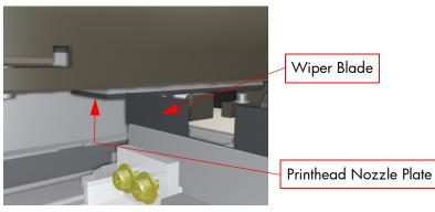
7 While holding the Wiper Blade in position, tighten the two screws that you loosened in a previous step.
