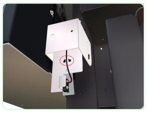
**6.** Cut the cable tie that secures the Sensor Cable to the Bracket.
