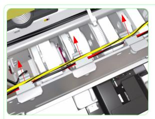
**10.** Release ALL the cables from the cable clips.
