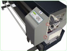
**6.** Remove two screws that secure the Right Subtank Cover to the Printer.
