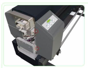
**6.** Remove two screws that secure the Left Subtank Cover to the Printer.
