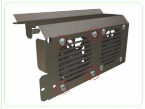
**13.** Remove four screws that secure the Printhead Cooling Fan to the Printhead Cooling Fan Assembly.
