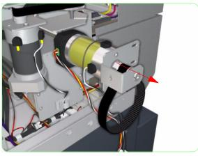
**10.** Remove the Paper-Axis Motor Assembly from the Printer.
