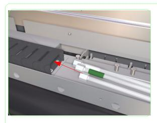
**43.** Thread the *narrow ends* of remaining three tubes through the other end of the cable carrier.
