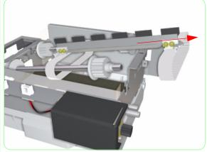
**13.** Remove the Wiper Blade and belts from the Wiping Station.
