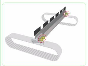
**14.** Remove four screws that secure the Wiper Blade to the Wiper Belts.
