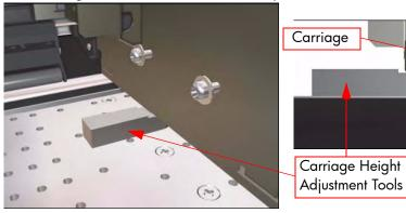
6 Insert the Carriage Height Adjustment Tools (square end) under the front part of the Carriage (both sides) until the second step.
