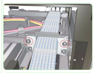
**13.** Remove the two screws that are used to secure the cable bracket to the carriage.
