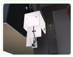
**4.** Turn the Waste Bottle Bracket 180 degrees so that you can access the Waste Bottle Sensor and Cable.
