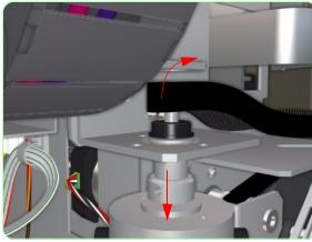
**10.** Release the Scan-Axis Belt and remove the Scan-Axis Motor from the Printer.
