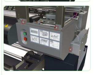
**4.** Remove three screws that secure the Lower Wiping Cover to the Printer.
