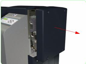
**2.** Remove the Upper Side Cover from the Printer.
