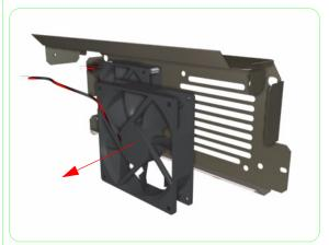
**14.** Remove the Printhead Cooling Fan from the Printhead Cooling Fan Assembly.
