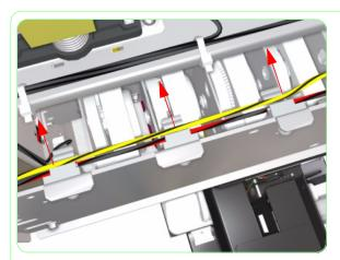
**8.** Release ALL the cables from the cable clips.
