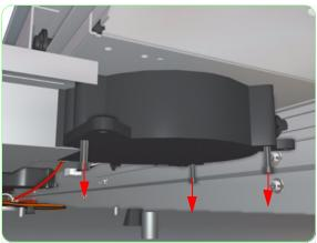
**3.** Remove 3 screws that secure the Vacuum Fan to the Printer.
