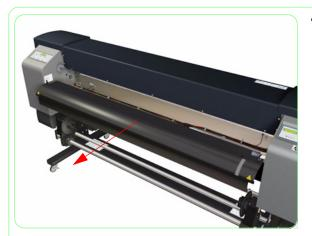
**4.** Remove the Front Heater from the Printer.
