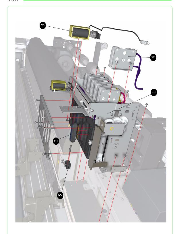
Figure 11: Capping Assemblies
