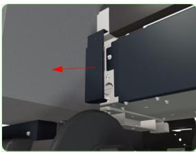
2. Remove the Left Electronics Module Side Trim from the Printer.
