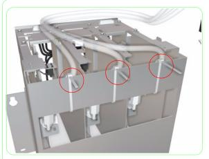
**53.** Attach three Insulock ties to ensure that the tubes remain in an upright positions, and then snip away the extra length of the Insulock ties.
