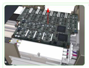
**13.** Remove the Carriage PCA from the Printer.
