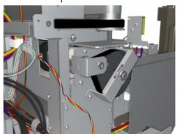
**2** Loosen three screws that secure the Paper-Axis Motor Bracket to the Printer.
