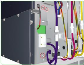
**7.** Remove the three screws that are used to secure the Ink Pump Assembly to the Printer.
