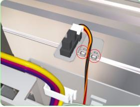
**5.** Remove the Home Position Sensor from the Printer.
