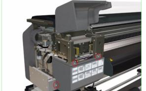
**4.** Remove three screws that secure the Lower Capping Cover to the Printer.
