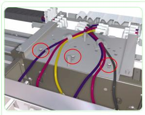
**19.** Remove the three screws that are used to secure the bracket assembly to the headbase.
