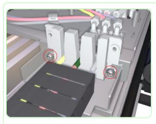
**19.** Remove the two screws used to secure the cable carrier to the guide bracket and carriage.
