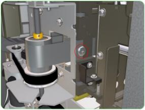
**4.** Remove one screw that secures the Belt to the left side of the Carriage Assembly.
