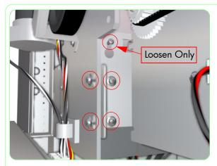
**28.** Loosen one screw (from the top) and four screws that secure the Capping Station.
