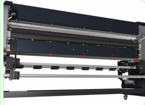
**5.** Loosen 5 screws that secure the Electronics Module Cover to the Printer.
