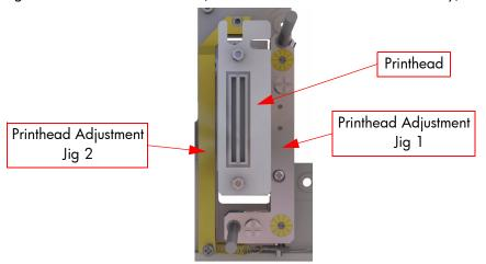
**8** Once the Printhead Adjustment Jigs are in place, tighten the front screw that secures the Printhead to the Carriage Base Plate.
