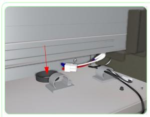
**5.** Pass the Heater Relay Cable through the hole in the Electronics Module.
