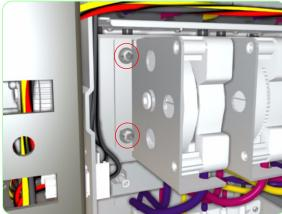
**15.** Remove two screws that secure the Prime Assembly to the Capping Station.
