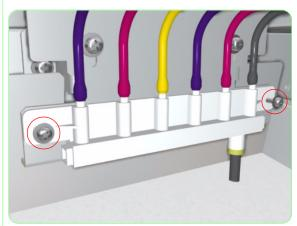
**30.** Remove two screws that secure the Capping Tubes Bracket to the Capping Station.
