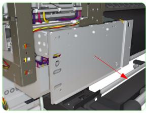
**12.** Remove the metal plate from the chassis.
