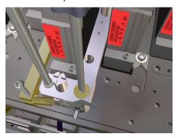
**6** Tighten the front screw that secures the Printhead to the Carriage Base Plate.
