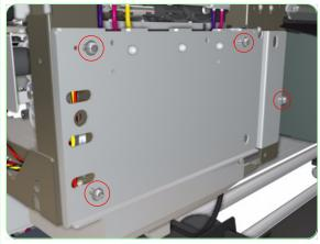
**10.** Remove four screws that secure the metal plate to the chassis.
