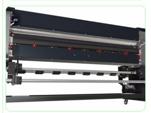
**6.** Remove six screws that secure the Electronics Module Cover to the Printer.
