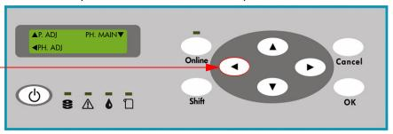
3 In the Printhead Adjustment submenu, scroll to "PH Voltage" and press the ▶ key.
