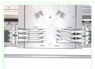
**46.** Connect the tubes at the Carriage PCA. Push or pull the tubes as necessary to connect them.
