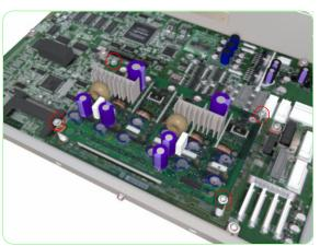
**7.** Remove four screws that secure the Head Relay Board to the Main PCA.
