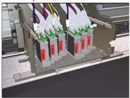
**9** With the Carriage Height Tools still in position, tighten the three screws that secure the Carriage base to the main Carriage Assembly. Tighten the left screw first, then the right screw, and then the middle screw.
