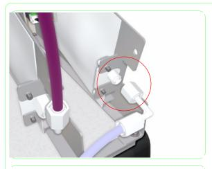
**33.** Loosen the plastic nuts and disconnect the subtank tubes from the subtank.
