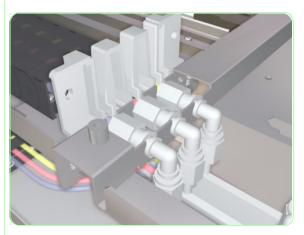
**18.** Loosen the plastic nuts and disconnect the three tubes where they connect at the guide bracket. (Steps 18 - 30 apply to both sides of the printer.)
