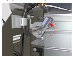
4 Loosen two screws that secure the Wiping Station on the right hand side.
