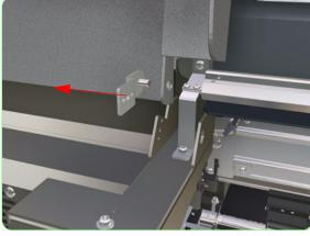
**3.** Remove the Hinge from the Printer.
