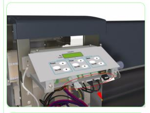
**5.** Loosen two screws that secure the Heater Panel to the Printer.
