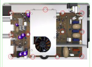
**7.** Remove 13 screws that secure the Power Supply Unit to the Support Tray.
