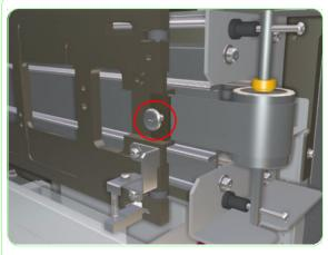
**22.** Remove the screw that is used to secure the belt to the right side of the Carriage Assembly.
