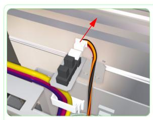
**6.** Disconnect the Cable from the Home Position Sensor.
