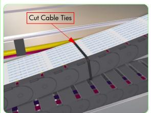
**15.** Cut ALL cable ties that secure the Trailing Cable to the Ink Tubes.
