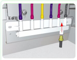
**31.** Disconnect the Waste Tube to the Capping Tubes Bracket.
