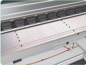
**3.** Remove 35 screws that secure the Center Platen to the Printer.
