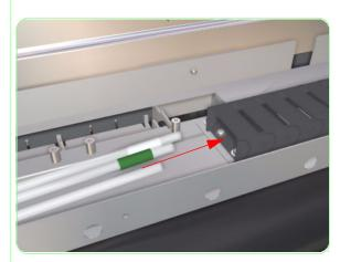
**40.** There is a narrow end and a wide end to each supply tube. Thread the *narrow ends* of three tubes through one end of the cable carrier.
