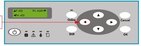
1 In the Printhead Adjustment submenu, scroll to "PH Adj Prints" and press the OK key.
