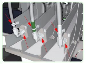
**56.** Connect the subtank tubes to the front of the capping-side subtank, and then attach three Insulock ties to ensure that the tubes remain in an upright positions. Snip away the extra length of the Insulock ties.
