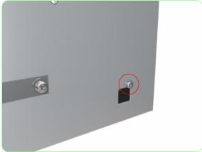
**3.** Remove one screw that secures the USB Connector to the Printer.
