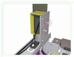
**15.** Remove two screws that secure the Solenoid Assembly to the Capping Station.
