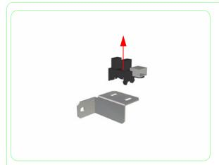
**5.** Remove the Media Lever Sensor from the Bracket.
