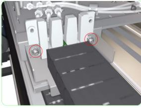
**49.** After securing the tubes, slide the carriage PCA back and forth along the length of the printer to ensure that the highest point of the cable carrier is the point at which the ends are attached to the carriage PCA.
