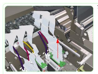
**7.** Disconnect the Printhead Connector Assembly from the Printhead and remove from the Printer.
