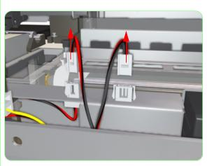
**7.** Release the Wiping Station cables from the cable clip.
