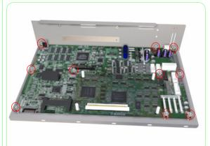
**9.** Remove 10 screws that secure the Main PCA to the Tray.
