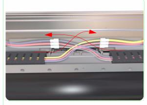
**34.** Pull the tubes out of the cable carrier in the direction shown.
