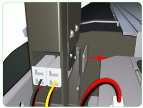
17. Remove the Sensor Plate from the Printer.
