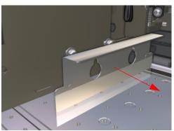
4 Make sure that the Printhead Height Lever is in the upper position (so that Printhead height is actually in the lower position). Make sure you loosen the two Printhead Height Adjustment screws before trying to change the position of the Printhead Height Lever and make sure you tighten the screws after changing the Printhead Height.
