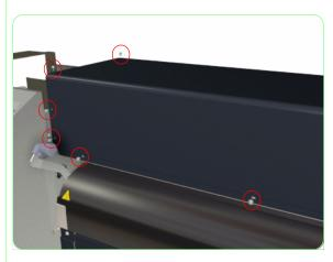
**5.** Remove seven screws that secure the Top Cover to the left hand side of the Printer.
