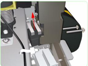
**15.** Remove two screws that secure the Right Rear Cover Sensor to the Chassis. Remove the Right Rear Cover Sensor.
