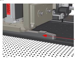
Carriage should sit on top of Step C
