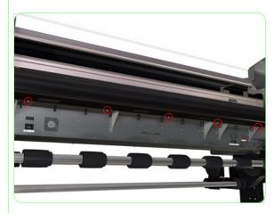
**1.** Remove five screws that secure the Rear Heater to the Printer.
