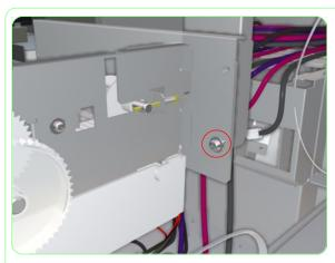
**14.** Remove one screw that secures the Wiping Station to the chassis.
