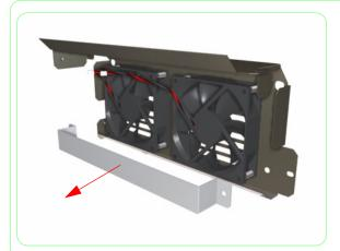
**12.** Remove the metal bracket from the Printhead Cooling Fan Assembly.
