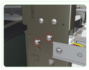
**16.** Loosen two screws that secure the Sensor Plate and the Left Rear Cover Sensor to the Chassis.
