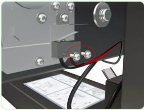
**5.** Remove two screws that secure the End-of-Media Sensor.
