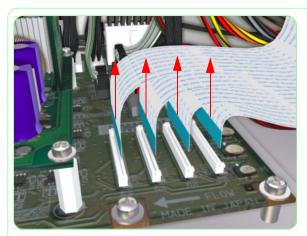
**16.** Disconnect the Trailing Cable from the Main PCA.
