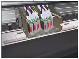
11 Insert the Carriage Height Tools again to check that the overall error is within +/- 0.2 mm. If the error exceeds this range, you will need to adjust the Carriage height again.
