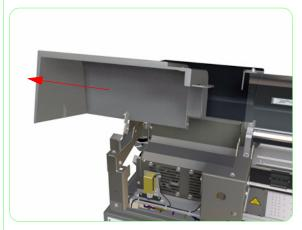
**4.** Slide the Capping Door to the left and remove from the Printer.
