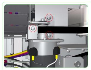
**6.** Loosen three screws that secure the Scan-Axis Motor Bracket to the Chassis.
