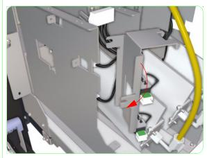
**14.** Remove the Subtank Sensors Assembly from the Subtank Station.
