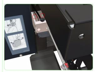
**3.** Remove two screws that secure the Waste Bottle Bracket to the Printer.
