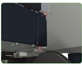
**4.** Remove the Right Electronics Module Side Trim from the Printer.
