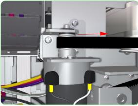
**7.** Move the Scan-Axis Motor Bracket to the right to release the tension on the Scan-Axis Belt.
