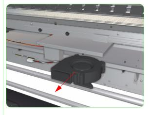
**4.** Remove the Vacuum Fan from the Printer.
