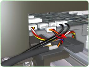
**3.** Disconnect the Line Sensor Cable from the Carriage PCA.
