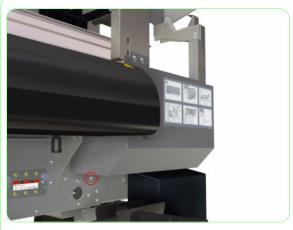
**5.** Remove one screw that secures the Lower Wiping Cover to the Printer.
