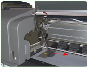
**6.** Remove the Line Sensor from the Printer.
