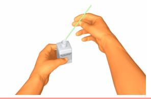
Make sure that you use the Cap Cleaning Liquid and NOT the Wiper Cleaning Liquid to clean the Capping Unit, otherwise you could cause damage to the Printheads.
