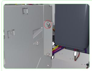
**6.** Loosen one screw from each side of the Subtank Station.
