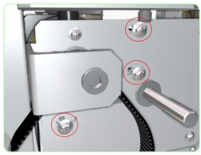
**9.** Remove three screws that secure the Paper-Axis Motor Bracket to the Chassis.
