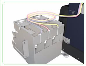
**37.** Remove the subtank and place it on the floor or on a bench.
