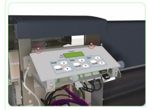
**6.** Remove two screws that secure the Heater Panel to the Printer.
