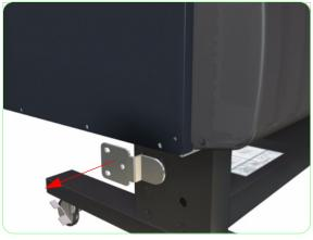
2. Remove the Hinge from the Printer.
