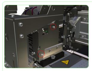
**6.** Remove two screws that secure the Printhead Cooling Fan Assembly to the Carriage Assembly.
