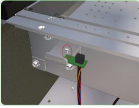
**3.** Remove one screw that secures the Rear Media Sensor to the Bracket.
