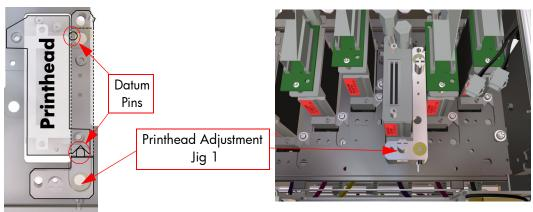
3 Insert the two Printhead Positioning Pins into the Printhead Adjustment Jig 1.
