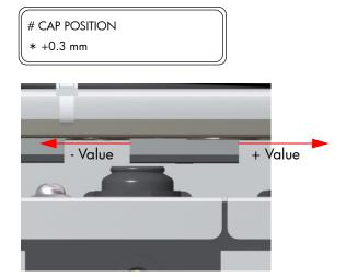
The value of the Cap Position should never be set as 0.0 mm as this means that the Cap Position has not been adjusted and will not work.
