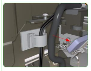
**4.** Release the Line Sensor Cable from the cable clip.
