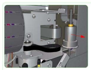
**8.** Release the Scan-Axis Belt and remove the Drive Pulley from the Printer.
