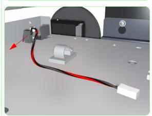
**7.** Remove the IC Door Sensor from the Ink Supply Station.
