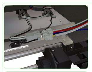
**4.** Disconnect the Rear Heater Cable from the Rear Heater.
