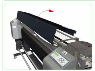
**6.** Remove the Top Cover from the Printer.
