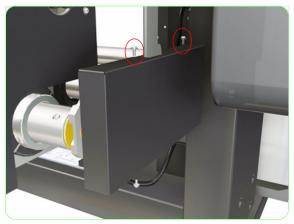
**3.** Remove two screws that secure Roll Module Cover.
