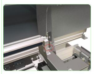
**1.** Remove one screw that secures the Wiping Door hinge to the Printer.
