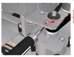
Hook the Push/Pull Gauge onto this hole
