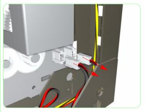
**18.** Disconnect the Capping Station cables.
