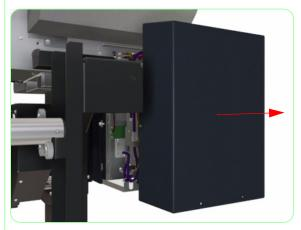
**3.** Remove the Rear Ink Cartridge Cover from the Printer.
