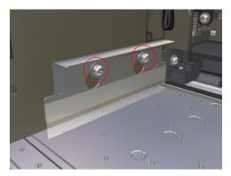
**3** Adjust the Carriage Shield so that there is a 2-3 mm clearance between the Carriage Shield and the Center Platen.
