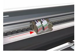
2 Remove the Carriage Shields from both sides of the Carriage Assembly.
