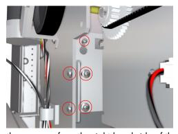
**4** Loosen three screws from the right hand side of the Capping Station.
