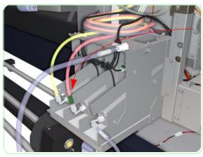
**30.** When the top part of the tube has drained, pull the tube through to the front side of the printer and continue to drain the tube into the waste bottle.
