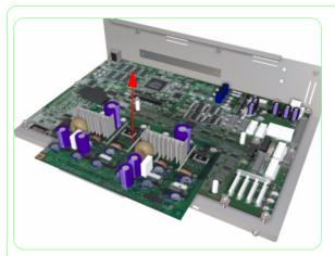
**8.** Remove the Head Relay Board from the Main PCA.
