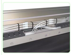
**42.** Secure the tubes using the two twist-ties.
