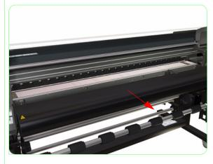
3. Pull out the Rear Heater slightly.
