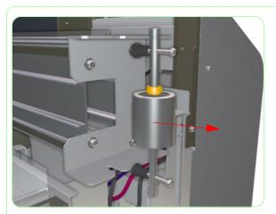
**11.** Remove the Tension Pulley from the Printer.
