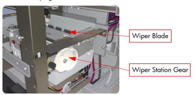
**5** Check that the center of the Wiper Blades are aligned with the center of the Printheads.
