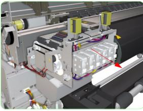
**32.** Remove the Capping Station from the Printer.
