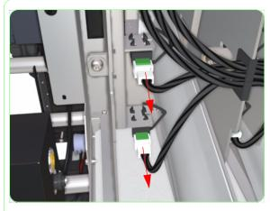
12. Disconnect the Subtank Sensor cables.
