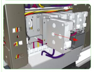
**16.** Remove the Prime Assembly from the Capping Station.
