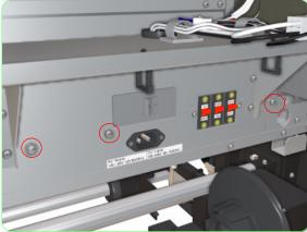
**3.** Remove three screws that secure the Heater Relay Assembly to the Printer from the rear.
