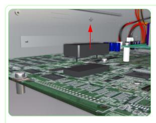
**11.** Pull up and remove the NVRAM from the Main PCA.
