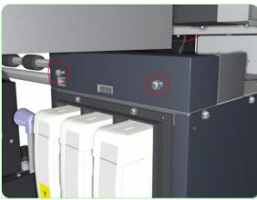
**3.** Remove two screws that secure the metal cover to the Ink Supply Station.
