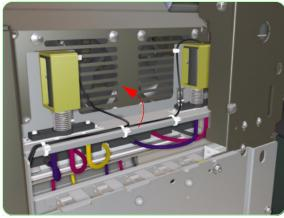
**11.** Rotate the Solenoid Assembly so that the Right Rear Cover Sensor can be accessed.
