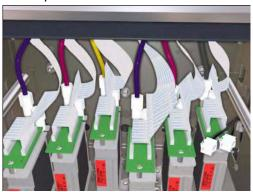
**8** Lower the Carriage onto the Carriage Height Tools that you inserted in the previous steps.
