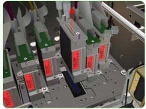
**11.** Remove the Printhead from the Carriage Assembly.
