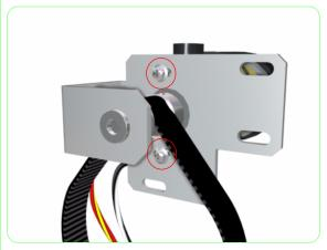
**11.** Remove two screws that secure the Bracket to the Paper-Axis Motor.
