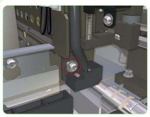
**5.** Remove one screw that secures the Line Sensor to the Carriage PCA.
