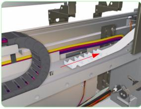
**20.** Remove the Trailing Cable from the Printer.
