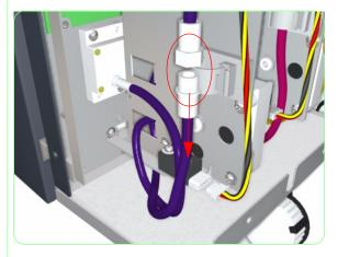
**5.** Carefully disconnect the Ink Pump Tube where it is attached with the plastic collar.
