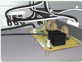
**6.** Disconnect ALL the cables from the Heater Relay Assembly.
