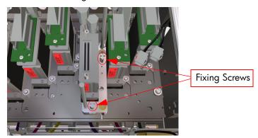
**5** Install the Printhead Adjustment Jig 2 in to position against the Carriage Base Plate.
