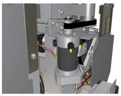
2 Loosen three screws that secure the Scan-Axis Motor Bracket to the Printer.
