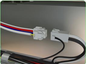
**3.** Disconnect the Front Heater Cable from the Front Heater.
