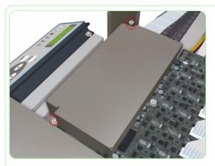
10. Remove two screws that secure the Carriage PCA Cover to the Carriage Assembly.
