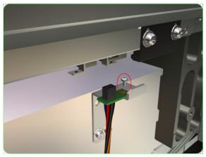
**4.** Remove one screw that secures the Front Media Sensor to the Bracket.
