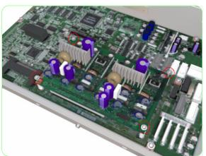
**7.** Remove four screws that secure the Head Relay Board to the Main PCA.
