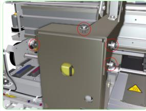
**23.** Remove four screws that secure the Right Capping Frame at the top.
