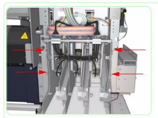
**36.** Loosen the top two screws and remove the bottom two screws that are used to secure the subtank to the printer.
