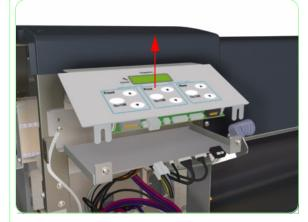
**7.** Remove the Heater Panel from the Printer.
