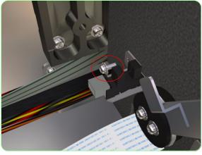
**3.** Remove one screw that secures the Media Lever Sensor to the Bracket.
