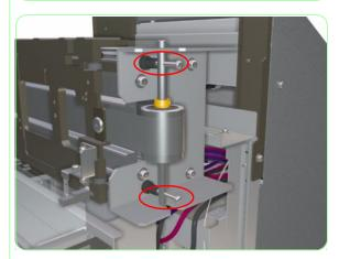
21. Loosen the two screws that are used to secure the Tension Pulley on the right side of the printer. Loosening these two screws will release the tension on the Carriage Belt. You must always loosen the belt before removing it.
