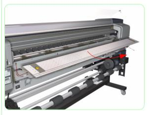
4. Remove the Center Platen from the Printer.
