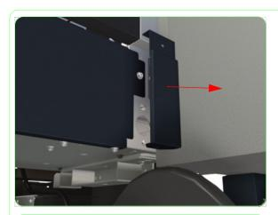
**4.** Remove the Right Electronics Module Side Trim from the Printer.
