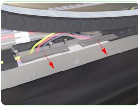
17. Remove the tube-holder brackets.
