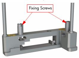
Place the Printhead Adjustment Jig on a flat surface and without holding it, gently turn the Adjustment Screws clockwise until the Printhead Adjustment Jig begins to move. Check that the Datum Pins touch the walls of the Printhead Adjustment Reference Plate. Do NOT force the Adjustment Screws too much as this could damage the Datum Pins.
