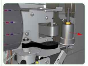
**8.** Release the Scan-Axis Belt and remove the Drive Pulley from the Printer.
