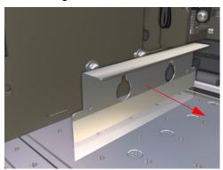
3 Make sure that the Printhead Height Lever is in the **upper** position (so that Printhead height is actually in the **lower** position). Make sure you loosen the two Printhead Height Adjustment screws before trying to change the position of the Printhead Height Lever and make sure you tighten the screws after changing the Printhead Height.
