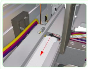
**19.** Pass the Trailing Cable through the hole (as shown in the drawing).
