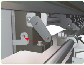
**10.** Release the Linkage from the Pinchwheel
