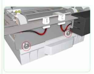
**8.** Unclip the Wiper Cleaning Assembly from the Wiping Station Assembly.
