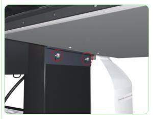
**8.** Remove two screws that secure the lnk Supply Station to the Printer.
