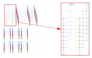
**2** Using a Measuring Loupe, you must first measure the deviation of the Printhead in the vertical position.
