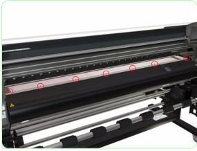
**2.** Remove seven screws that secure the Rear Heater to the Printer.
