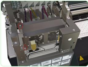
**7.** Remove two screws that secure the Printhead Cooling Fan Assembly to the Carriage Assembly.
