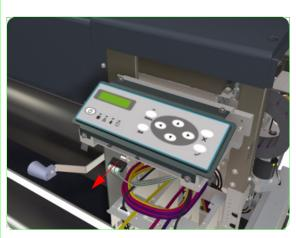
**5.** Loosen two screws that secure the Front Panel to the Printer.
