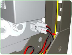
**13.** Disconnect the Solenoid Assembly cable.
