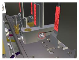
**9** Remove the tube cap from the Printhead.
