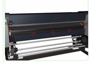
**1.** Remove seven screws that secure the Front Heater to the Printer.
