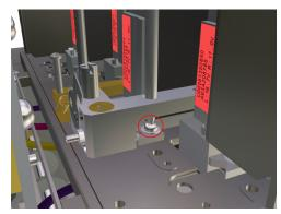
10 Using the measurement obtained in step 8, calculate how many scales you will need to turn the Slant Adjustment Screw to adjust the slant position of the Printhead.
