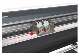
5 Insert the Carriage Height Adjustment Tools (round end) under the rear part of the Carriage (both sides) until the third step.
