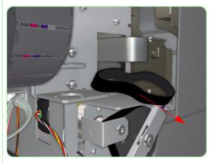
11. Remove the Scan-Axis Belt from the Printer.
