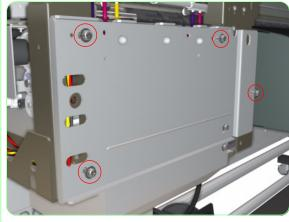
**11.** Remove four screws that secure the metal plate to the chassis.
