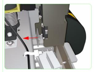
14. Remove the Sensor Plate from the Printer.
