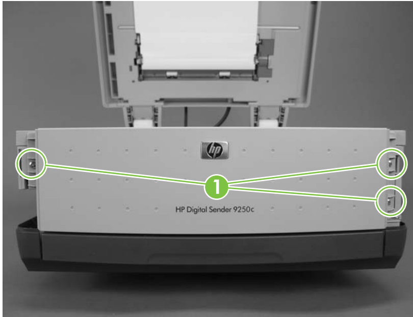
Figure 5-52 Removing the scanner front cover
