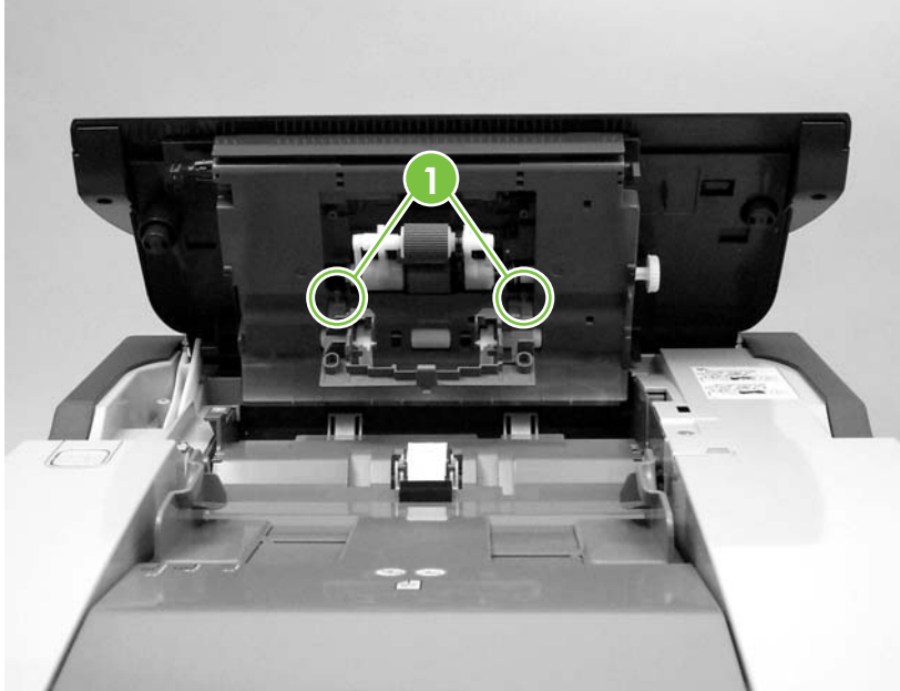
Figure 5-6 Removing the pickup-roller cover (2 of 2)
