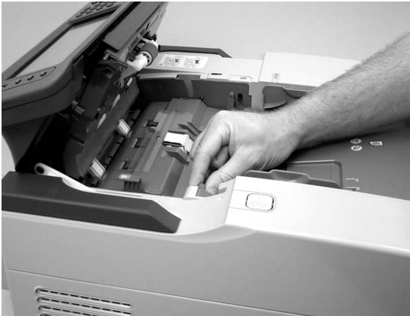
Figure 5-26 Removing the paper input tray (2 of 2)
