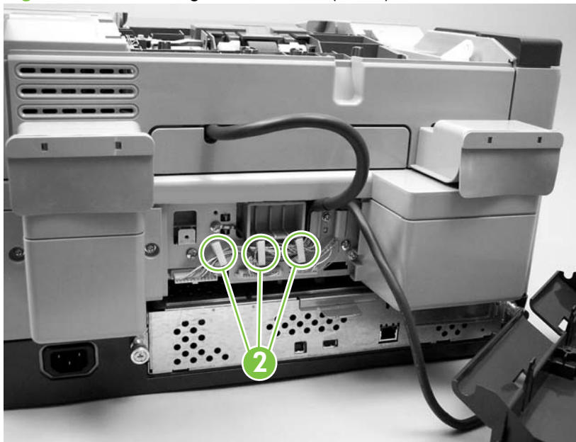
Figure 5-68 Removing the ADF cable (2 of 5)
