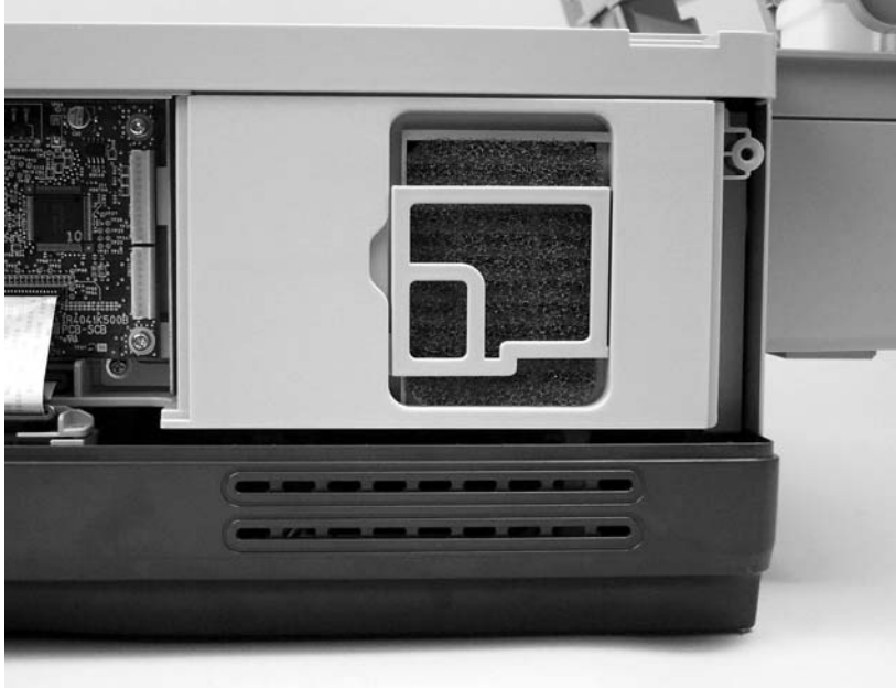
Figure 5-66 Removing the fan filter
