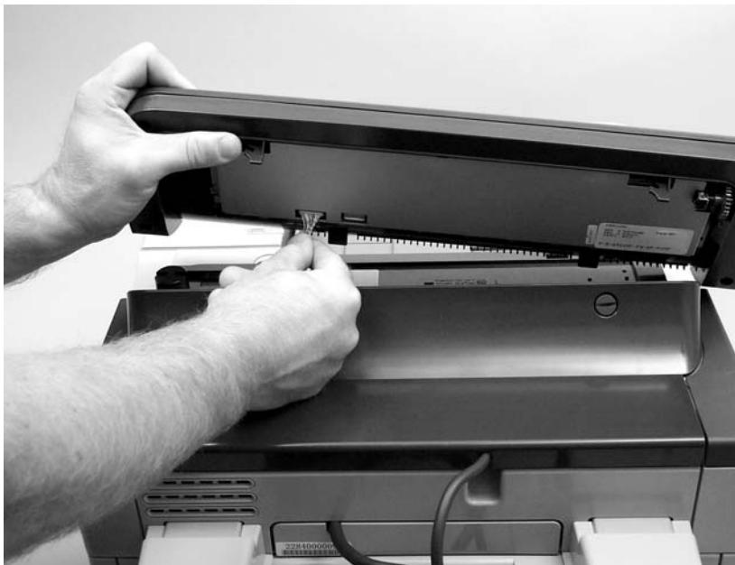
Figure 5-16 Removing the control panel (2 of 2)
