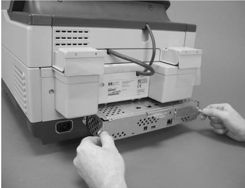
Figure 5-18 Removing the formatter cage
