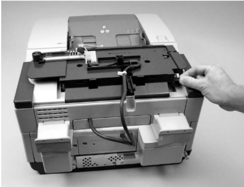
Figure 5-35 Removing the control-panel cover assembly (4 of 6)
