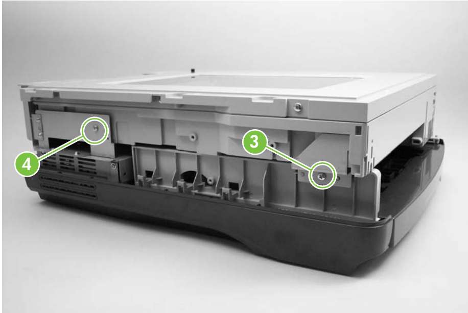
Figure 5-79 Removing the flatbed scanner assembly (2 of 4)
