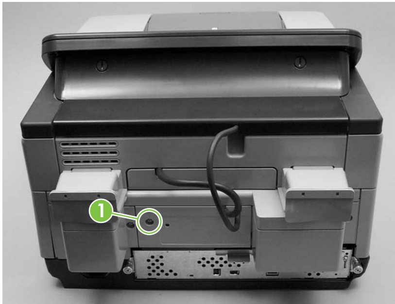
Figure 5-53 Removing the scanner rear cover
