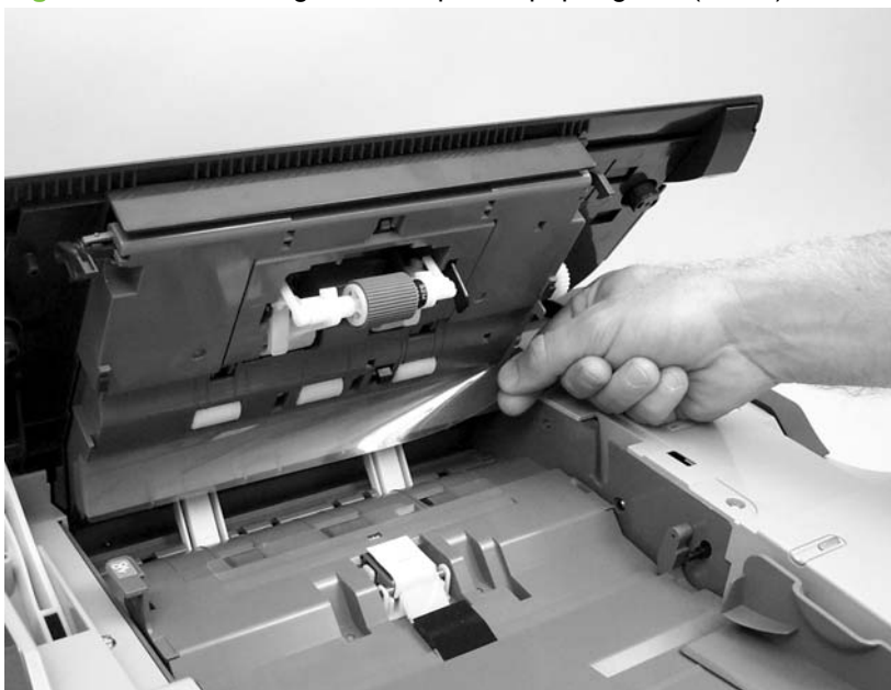
Figure 5-74 Removing the clear plastic paper guide (2 of 2)
