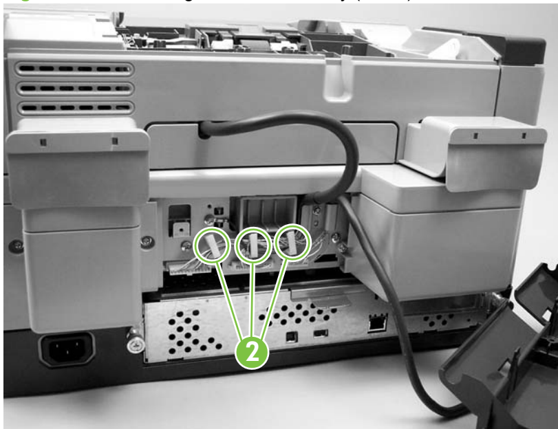
Figure 5-58 Removing the ADF assembly (2 of 3)
