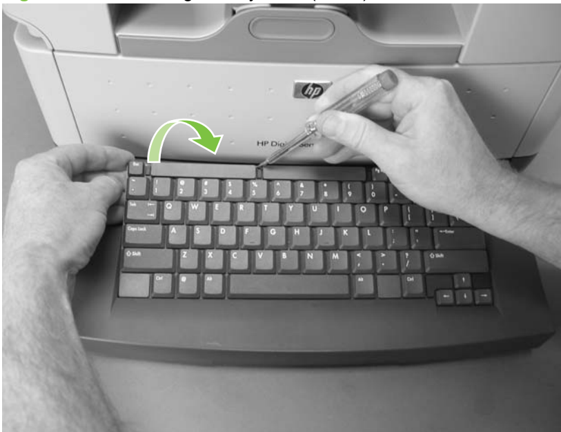
Figure 5-28 Removing the keyboard (2 of 3)
