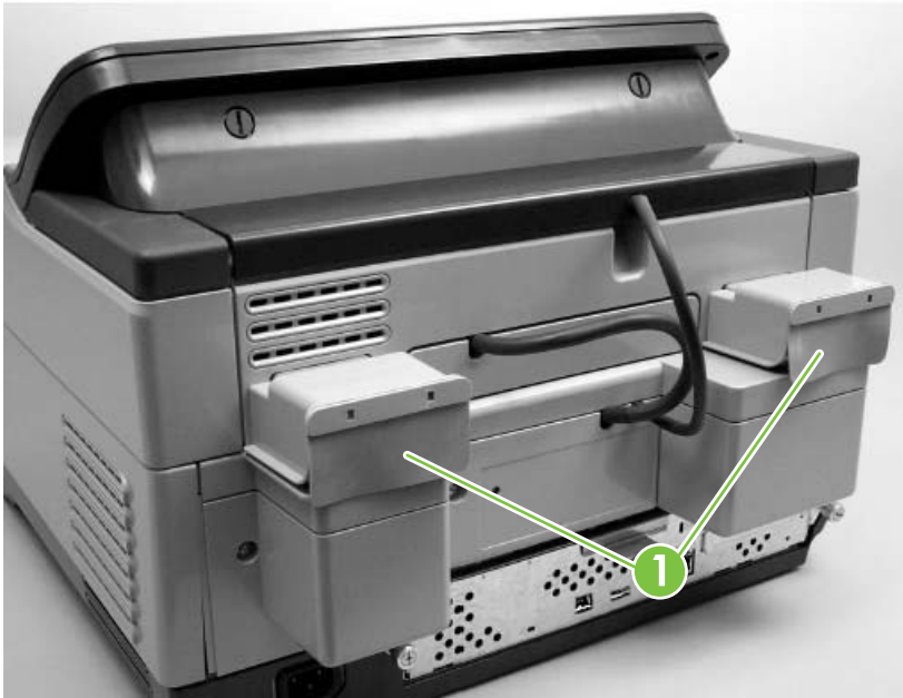
Figure 5-24 Removing the hinge flaps
