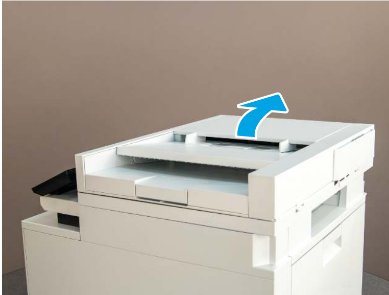
Figure 5-1 Open the cover
