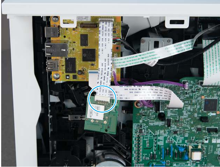
Figure 5-250 Remove the PCA
