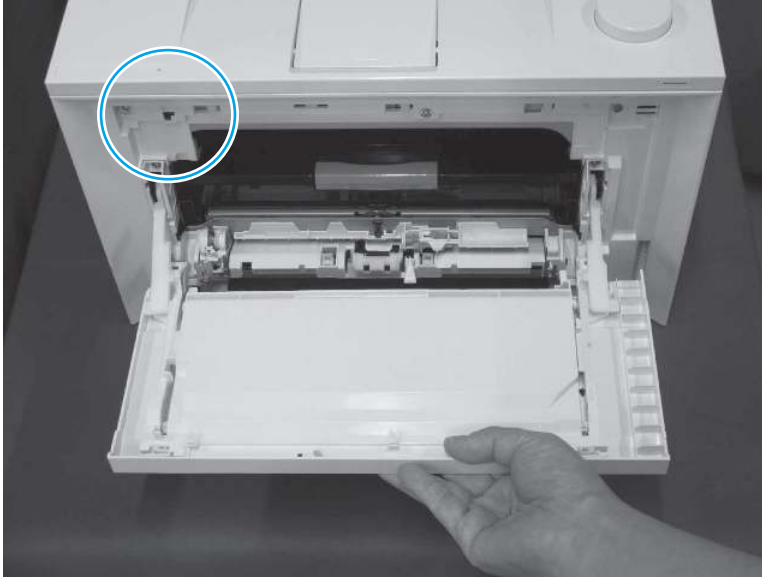
Figure 4-38 Defeat the cartridge door interlock
